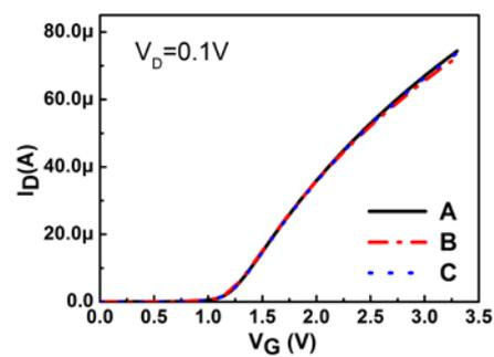
Fig.3  $I_D$ - $V_G$  curves of devices with various depths in Si recess.
