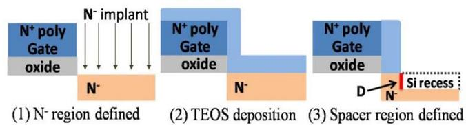
Fig. 2 Schematic process flow that leads to Si recess structure.
