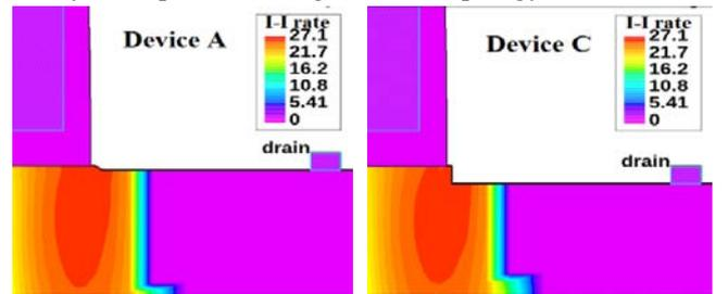
Fig. 7 I-I rate contour of devices A and C bias at stress condition.
