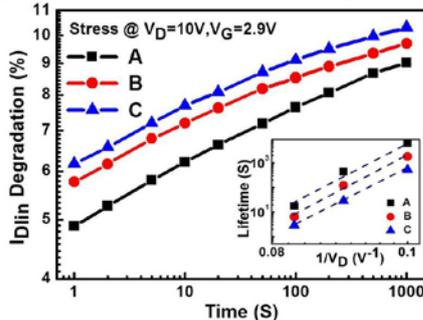
Fig. 6  $I_{Dlin}$  degradation of devices under hot-carrier stress. Hot-carrier lifetime vs.  $1/V_D$  is shown in the inset.
