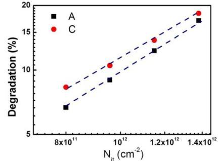
Fig. 8 The impact of hot-carrier induced  $N_{it}$  on  $I_{Dlin}$  degradation.
