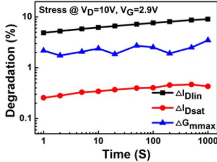
Fig. 5  $I_{Dlin}$ ,  $I_{Dsat}$ , and  $G_{mmax}$  degradation of device A under hot-carrier stress.
