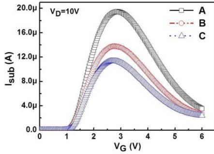
Fig. 4  $I_{sub}$ - $V_G$  curves of devices with various depths in Si recess.
