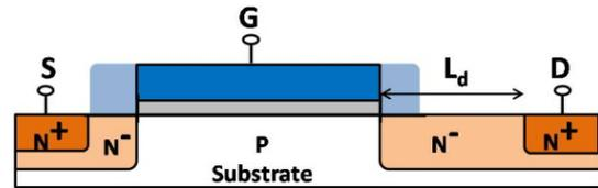
Fig. 1 Schematic cross section of the device used in this paper.
