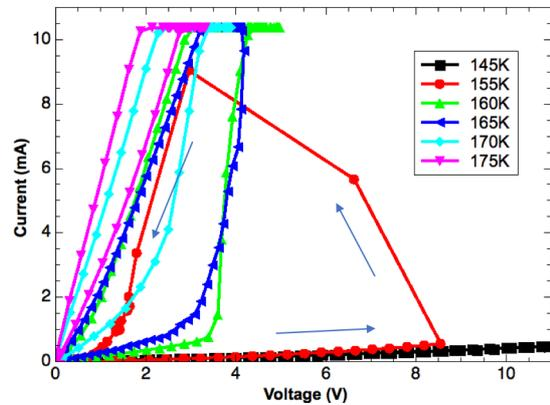
Fig. 3 Resistance switching of a  $100 \times 1 \mu\text{m}^2$  bridge induced by a voltage pulse: Current vs voltage at fixed temperatures between  $145\text{K}$  and  $175\text{K}$
