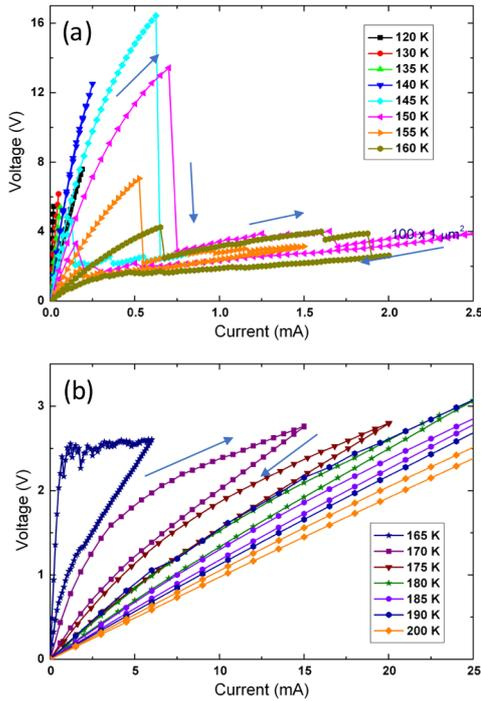
Fig. 2 Resistance switching of a  $100 \times 1 \mu\text{m}^2$  bridge induced by current sweep: Voltage vs current at different temperatures. The arrows indicate the direction of current sweep.
