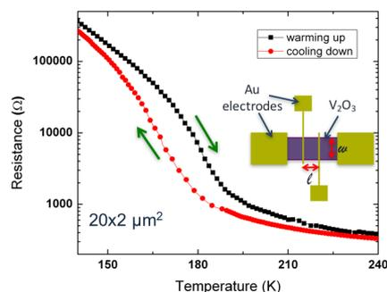
Fig. 1 Resistance vs temperature of a  $20 \times 2 \mu\text{m}^2$  microbridge.
