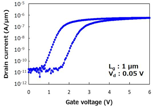
Fig. 5. Measurement results of  $I_d$ - $V_g$  characteristics of the SONOS memory with conventional FET structure.
