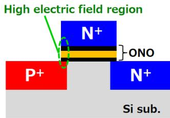
Fig. 1. Schematic of the cross-section of a SONOS memory cell with TFET structure.
