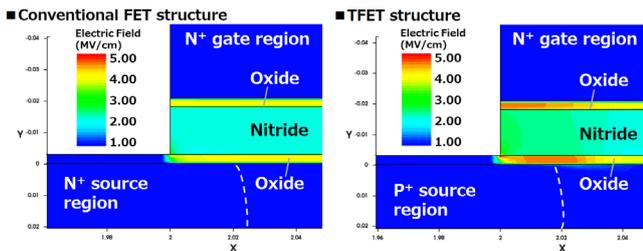
Fig. 2. TCAD simulation results of electric field distributions of SONOS memory devices with conventional FET structure (left) and TFET structure (right).
