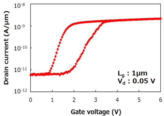
Fig. 6. Measurement results of  $I_d$ - $V_g$  characteristics of the SONOS memory with TFET structure.
