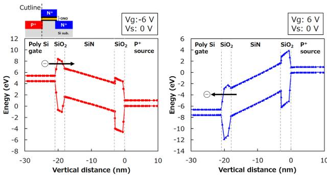
Fig. 3. Energy band diagram of the overlap region between gate and source of the SONOS memory with TFET structure for programming (left) and erasing operation (right).
