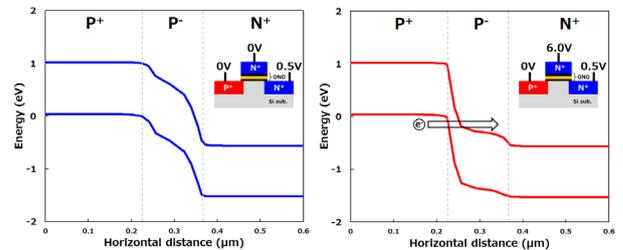
Fig. 7. Energy band diagram along the channel region of the SONOS memory with TFET structure at OFF state (left) and ON state (right).
