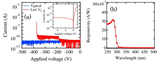
Fig. 5. (a)  $I$ - $V$  characteristics of the Pt/ $Mg_xZn_{1-x}O$ /ZnO SBD in reverse bias voltage. The inset shows the low voltage-range characteristics, (b) Spectral responsivity.
