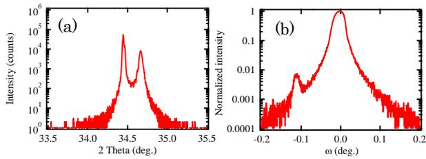
Fig. 3. (a) 2Theta-Omega scan of ZnO (0002) and  $Mg_xZn_{1-x}O$  (0002), (b)  $Mg_xZn_{1-x}O$  (0002) rocking curve.
