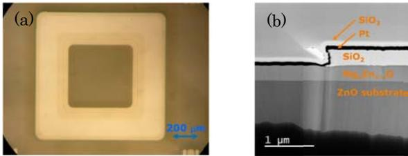
Fig. 4. (a) An optical microscope image of fabricated Pt/ $Mg_xZn_{1-x}O$ /ZnO SBD, (b) a TEM image of a cross-sectional view at the edge of the field plate portion.
