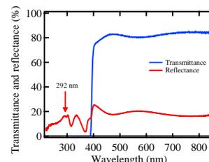
Fig. 2. Transmittance and reflectance spectra of the Mg<sub>x</sub>Zn<sub>1-x</sub>O film deposited on the ZnO substrate.
