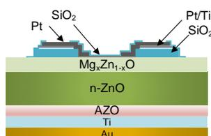
Fig. 1. Schematic cross-sectional view of the Pt/Mg<sub>x</sub>Zn<sub>1-x</sub>O/ZnO SBD.
