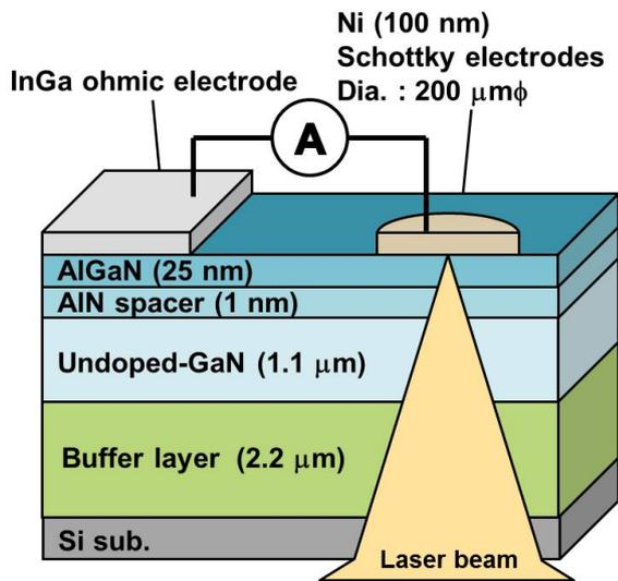
Fig. 1 Ni Schottky contacts formed AlGaIn/GaN HEMT structure grown on Si substrates. Because the incident visible laser beam was absorbed, the Si substrates were thinned to be about 30  $\mu\text{m}$  thick.
