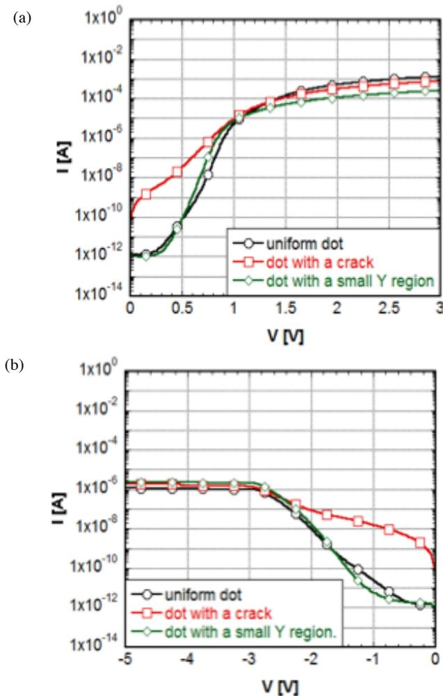
Fig. 3 (a) Forward and (b) reverse I-V characteristics of the Ni/AlGaIn/GaN Schottky contacts: (i) uniform, (ii) with a crack, and (iii) with a small Y region.
