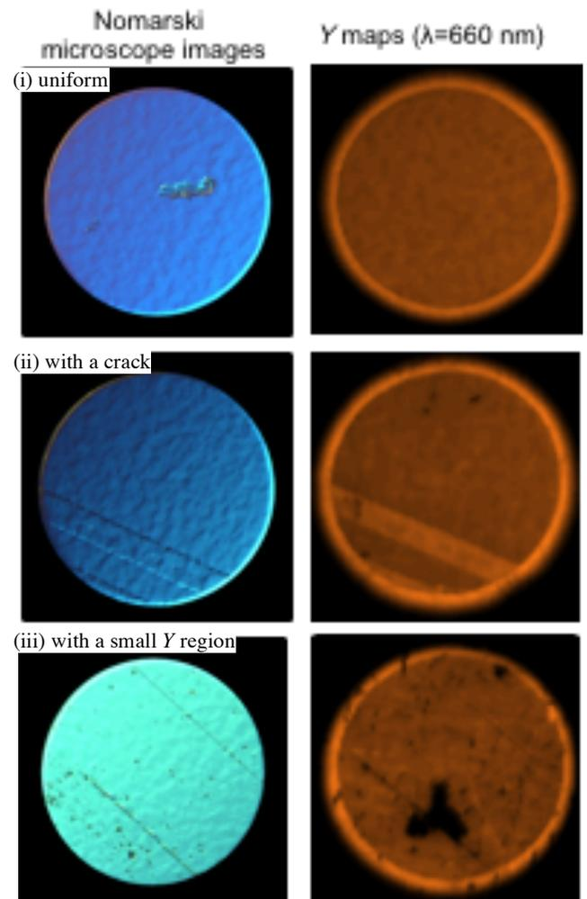
Fig. 4 Microscope images and Y maps at  $\lambda = 660 \text{ nm}$  of the same Ni/AlGaIn/GaN contacts as shown in Fig. 3.
