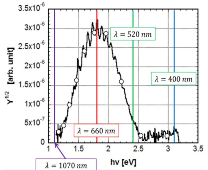
Fig. 2 Typical PR spectra of the Ni/AlGaIn/GaN Schottky contact. The signal was detected around  $\lambda = 660 \text{ nm}$ .
