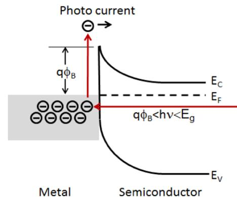
Fig. 2 Internal photoemission process in a metal/semiconductor interface.
