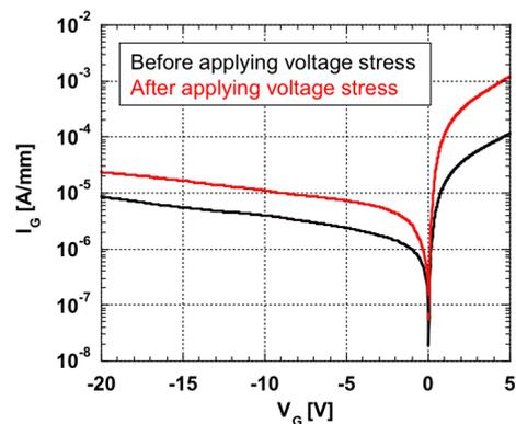
Fig. 5 Gate  $I$ - $V$  characteristics of the device shown in Fig. 4.
