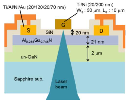
Fig. 1 AlGaN/GaN MIS HEMT structure grown on a sapphire substrate.
