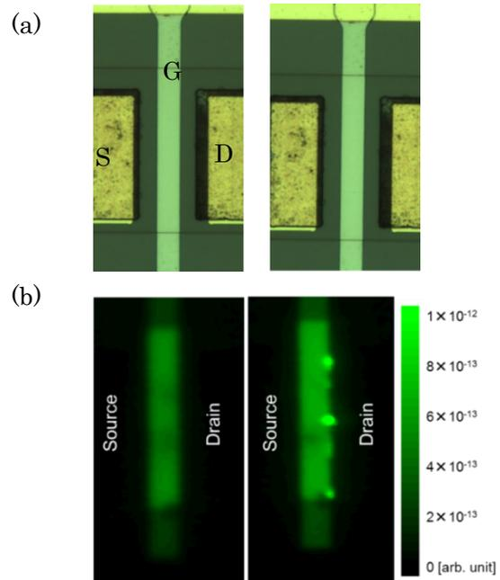
Fig. 4 (a) Optical microscope images and (b)  $Y$  maps without a bias voltage before and after the voltage stress conducted in the measurement shown in Fig. 3.
