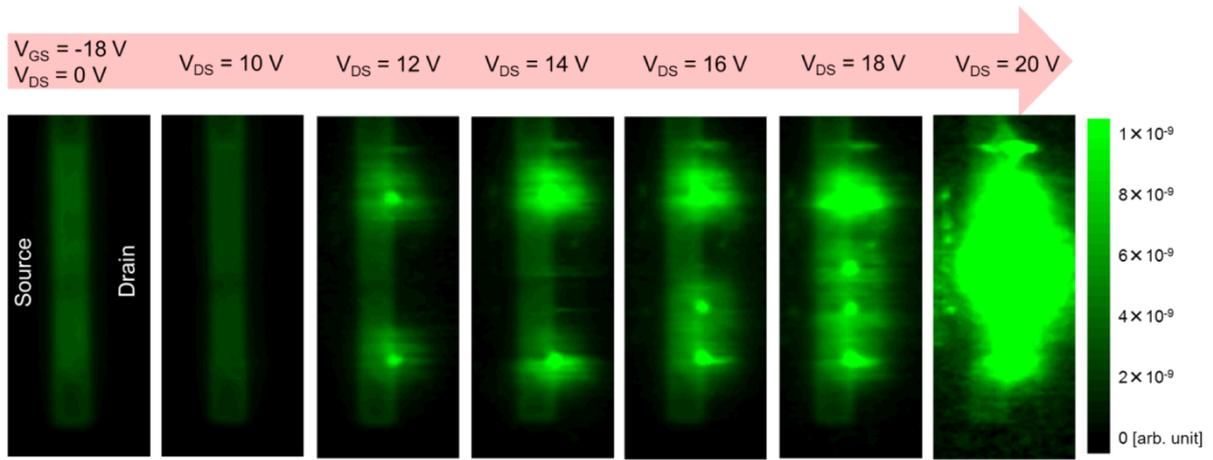
Fig. 3 Video-mode SIPM results for the gate electrode under the drain-gate stress voltage swept up to 20 V.
