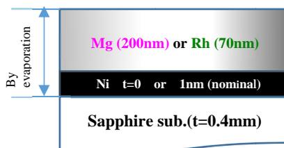
Fig.3.2.1 Structure of samples of Mg(200nm), Al(200nm), Ni/Mg(1nm/200nm), NiAl(1nm/200nm) and Rh(70nm)
