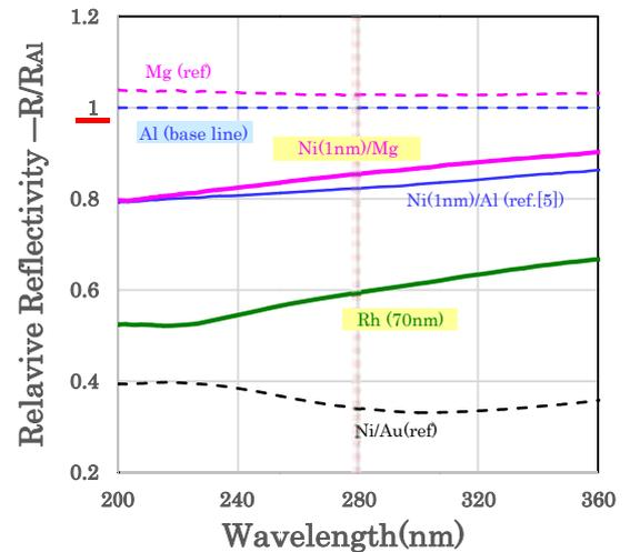
Fig.3.2.2 Reflectivity spectra of mirror samples. Two broken lines of purple and blue indicate mirrors of Mg and Al (base line) on sapphire substrate without Ni, respectively. Solid lines of purple, blue, green and black indicate mirrors of Ni(1nm)/Mg, Ni(1nm)/Al, Rh and Ni(20nm)/Au on sapphire substrate, respectively.
