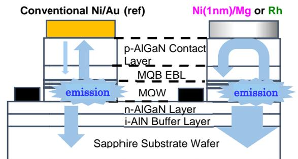
Fig.3.1.1 Structure of LED samples. Left-hand indicates the case of conventional Ni/Au p-electrode for reference and right-hand indicates the case of highly reflective p-electrode of Ni(1nm)/Mg and Rh.
