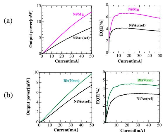
Fig.3.1.2 Characteristics of I-L (L/H) and I-EQE (R/H) of AlGaIn UVC LED with reflective p-type electrode of (a) Ni/Mg and (b) Rh, respectively
