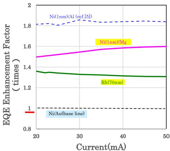
Fig.3.1.3 Dependency on reflective-p-electrode of EQE enhancement factor. Two solid lines of purple and green indicate case of Ni(1nm)/Mg and Rh, respectively. Two broken lines of blue and black indicate case of Ni(1nm)/Al and Ni/Au (base line), reflectively.
