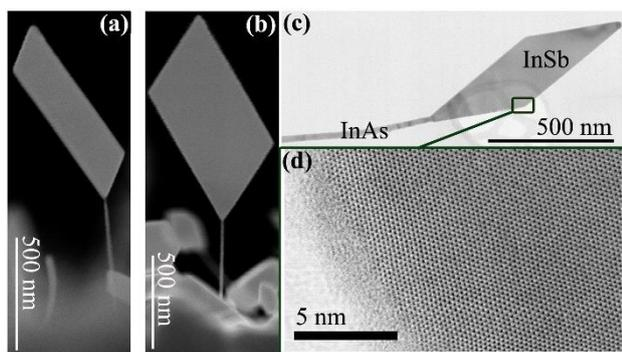
Fig. 2 SEM and TEM images of typical InSb nanosheets grown on InAs nanowire stems using Ag as catalysts by MBE.
