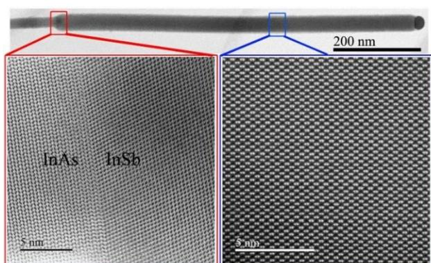
Fig. 1 TEM images of a typical InSb nanowire grown on InAs nanowire stem using Ag as catalysts.
