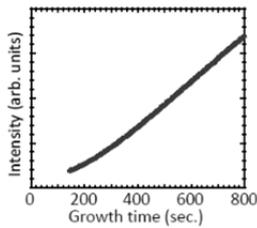
Fig. 3 Evolution of integrated intensity of GaInN (10-11) peak during growth.
