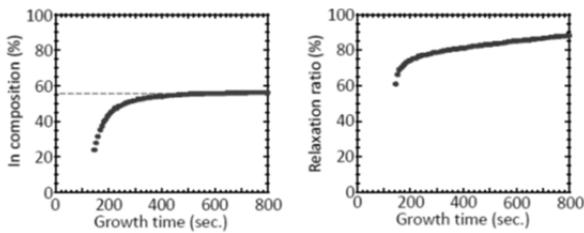
Fig. 2 Evolution of In composition and relaxation ratio of GaInN during growth.
