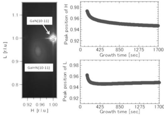
Fig. 1 One of RSM obtained in this study and evolution of peak position for (10-11) diffraction peak of GaInN as function of growth time.
