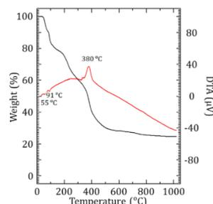
Fig.1 TG-DTA plots of Y(C<sub>5</sub>H<sub>7</sub>O<sub>2</sub>)<sub>3</sub>·nH<sub>2</sub>O
