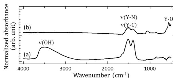
Fig.3 FT-IR patterns of yttrium oxide thin films (a) before and (b) after annealing
