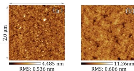
Fig.4 Surface morphology of yttrium oxide thin films: (a) before annealing and (b) after annealing
