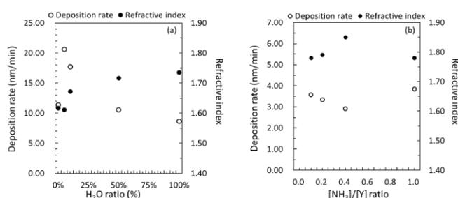
Fig.2 The deposition rate and refractive index of yttrium oxide thin films with (a) different H<sub>2</sub>O ratio and (b) different [NH<sub>3</sub>]/[Y] ratio
