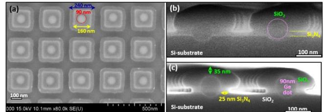
Fig. 1 Formation of Ge dots by the selective oxidation of SiGe nanopillars over buffer layer of Si<sub>3</sub>N<sub>4</sub> on SOI substrate. (a) Plan-view and cross-sectional SEM micrographs of SiO<sub>2</sub>/Ge dots/Si<sub>3</sub>N<sub>4</sub> heterostructure (b) following thermal oxidation and (c) released from Si<sub>3</sub>N<sub>4</sub>.
