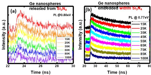
Fig. 4 Time-resolved PL decays for PL peaks at (a) 0.8eV and (b), 0.77eV measured from 60nm Ge dots embedded within  $Si_3N_4$  or not over temperatures ranging from 15–100K.
