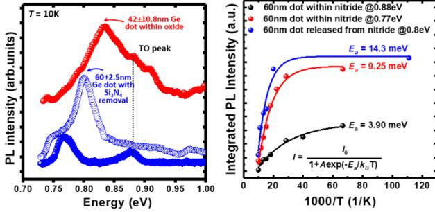
Fig. 3 (a) PL spectra measured at  $T = 10K$  on 60nm Ge QDs embedded within  $SiO_2$ , with  $Si_3N_4$  in close proximity and with  $Si_3N_4$  removal. (b) the Arrhenius plot of the integrated PL intensity at peak energy of 0.77eV and 0.8eV, respectively, for Ge nanodots embedded within  $Si_3N_4$  or not, respectively.
