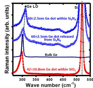
Fig. 2 Raman spectra of bulk Ge as well as Ge QDs embedded within a SiO<sub>2</sub>, Si<sub>3</sub>N<sub>4</sub>/SiO<sub>2</sub>, and released from Si<sub>3</sub>N<sub>4</sub> matrix.
