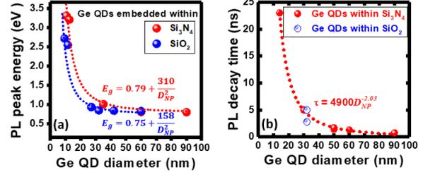
Fig. 5 Size-dependent (a) PL peak energy and (b) PL decay time of Ge QDs embedded within  $SiO_2$  and  $Si_3N_4$ .
