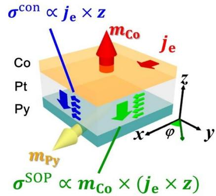
Figure 1: Schematic of Py/Pt/Co system. Two types of out-of-plane spin currents with different spin polarizations are generated by the electrical current injection.  $\mathbf{m}_{\text{Co}}$  and  $\mathbf{m}_{\text{Py}}$  correspond to the magnetization vector of the Co and Py layer respectively.
