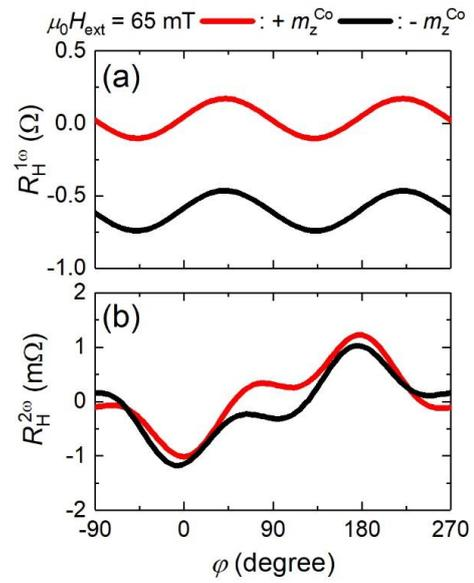
Figure 2: Angle-scan harmonic Hall measurement of Py/Pt/Co system. (a) First harmonic resistance Hall  $R_H^{1\omega}$  and (b) second harmonic Hall resistance  $R_H^{2\omega}$  measured under external field of 65 mT with  $+m_z^{\text{Co}}$  (red line) and  $-m_z^{\text{Co}}$  (black line) states.
