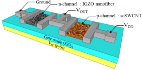
Fig. 2 Schematic structure of fabricated hybrid scSWCNT random network/IGZO nanofiber complementary inverters.
