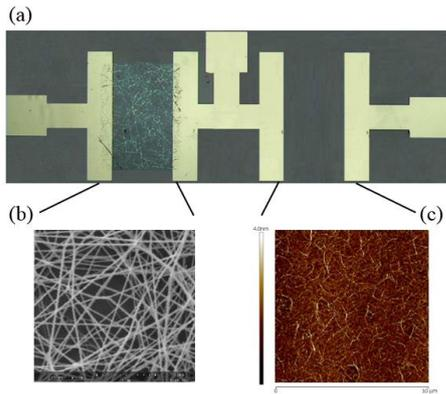
Fig. 3 (a) Optical microscope image of hybrid CMOS-type inverter. (b) SEM image of IGZO nanofibers in the n-channel region. (c) AFM image of scSWCNT network in the p-channel region.
