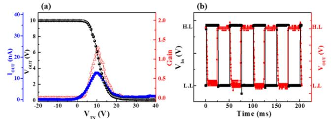
Fig. 5 (a)  $V_{out}-V_{in}$ , switching current and gain characteristics of inverter measured with  $V_{DD} = 10$  V, (b)  $V_{out}-V_{in}$  characteristics at input signal of 20 V square wave (20 Hz).
