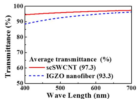
Fig. 1 Optical transmittance spectra of the IGZO nanofibers and scSWCNT random networks.
