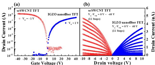
Fig. 4 (a) Transfer and (b) output characteristic curves of scSWCNT network and IGZO nanofiber FETs.
