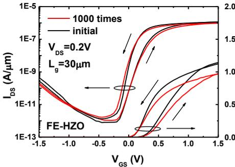
Fig. 4.  $I_{DS}V_{GS}$  of 5nm FE-HZO with multiple DC sweep (1000 times). The drain current and SS degradation is occurred.
