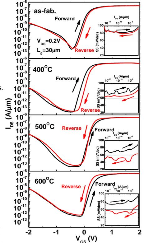
Fig. 3.  $I_{DS}V_{GS}$  of 5nm HZO for as-fab, and annealing at 400°C, 500°C & 600°C. The as-fab. 5nm HZO shows  $SS > 60 \text{ mV/dec}$  and positive  $V_T$  shift for reverse sweep, which is the typical dielectric high-K behavior. The counterclockwise direction of sweep and  $SS_{rev} < 60 \text{ mV/dec}$  is obtained due to NC effect after 600°C annealing.
