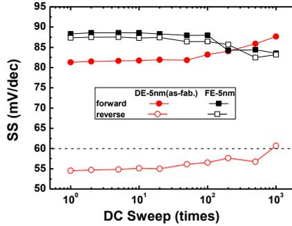
Fig. 5. SS of 5nm DE-HZO and FE-HZO with multiple DC sweep. The FE-HZO FET exhibits high sustainability until 100 times.
