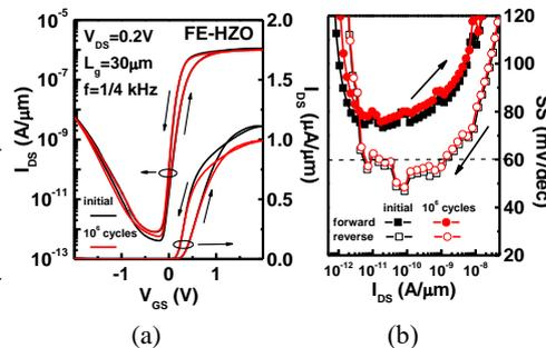
Fig. 17. (a)  $I_{DS}V_{GS}$  and (b) SS vs.  $I_{DS}$  of 5nm FE-HZO with AC stress cycles. There is no significant current degradation for 5nm FE-HZO FET after  $10^6$  cycles with frequency 1/4 kHz AC stress. The SS exhibits 40-60 mV/dec for initial and after AC stress.
