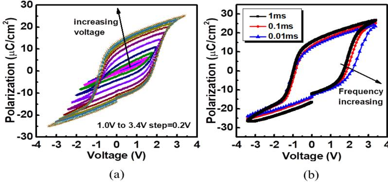
Fig. 2. The typical ferroelectric characteristics of MFM (metal/ferroelectric/metal) with HZO 10 nm. (a) Hysteresis loop with different applied voltage from 1V to 3.4V. (b) Hysteresis loop with different operation frequency. The related reliability discussion of ferroelectric HZO FET in this work is based on the typical characteristics.
