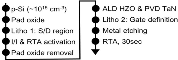
Fig. 1. The process flow of the baseline Ferroelectric HfZrO<sub>x</sub> FETs with gate-last process.
