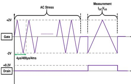
Fig. 6. AC stress with triangular waveform for periods 4ms. The stress voltage is bipolar  $\pm 2 \text{ V}$  to emulate fast sweep
