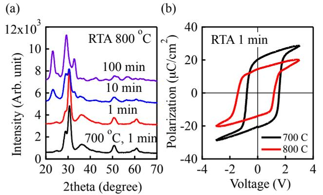
Fig. 2. 10-nm-thick  $\text{Hf}_{0.5}\text{Zr}_{0.5}\text{O}_2$  films annealed by RTA process at 700 °C and 800 °C. (a) GIXRD patterns and (b) P-V characteristics.
