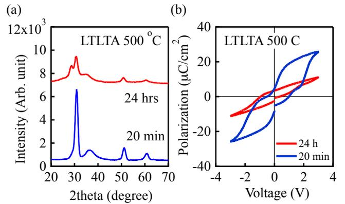
Fig. 4. 10-nm-thick  $\text{Hf}_{0.5}\text{Zr}_{0.5}\text{O}_2$  films annealed by LTLTA process at 500 °C. (a) GIXRD patterns and (b) P-V characteristics.
