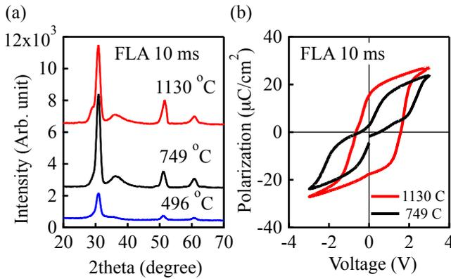
Fig. 3. 10-nm-thick  $\text{Hf}_{0.5}\text{Zr}_{0.5}\text{O}_2$  films annealed by FLA process at 496, 749, and 1130 °C. (a) GIXRD patterns and (b) P-V characteristics.
