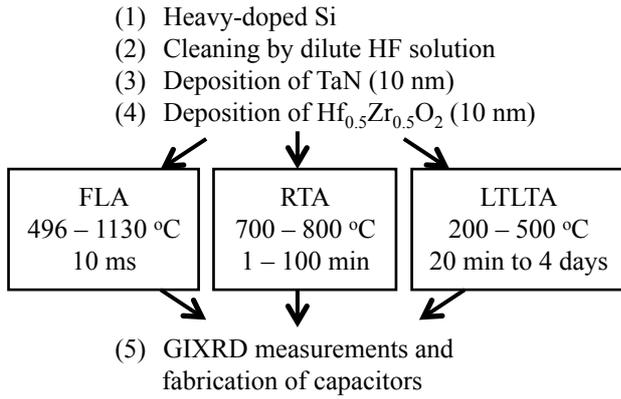
Fig. 1. Process flow to obtain crystalline films using flash lamp anneal (FLA), rapid thermal anneal (RTA), and low-temperature long-time anneal (LTLTA).
