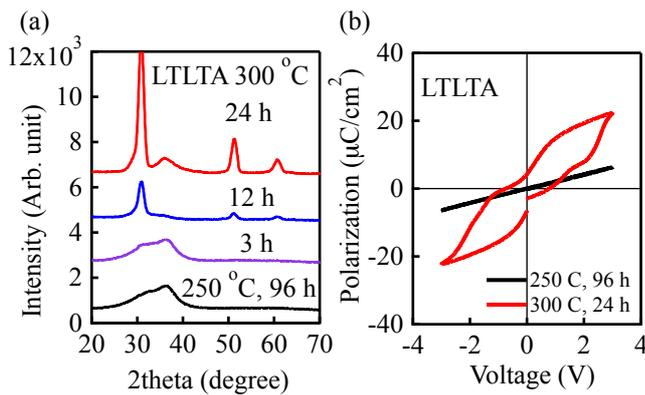
Fig. 5. 10-nm-thick  $\text{Hf}_{0.5}\text{Zr}_{0.5}\text{O}_2$  films annealed by LTLTA process at 250, and 300 °C. (a) GIXRD patterns and (b) P-V characteristics.
