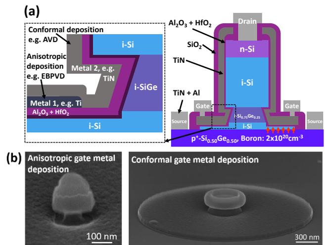
Fig. 1 (a) Device concept overview of a gate-normal TFET and zoom exemplifying the use of two gate metals. (b) SEM images illustrating the two-step self-aligned creation of a dual-metal gate utilizing anisotropic deposition followed by conformal metal deposition.
