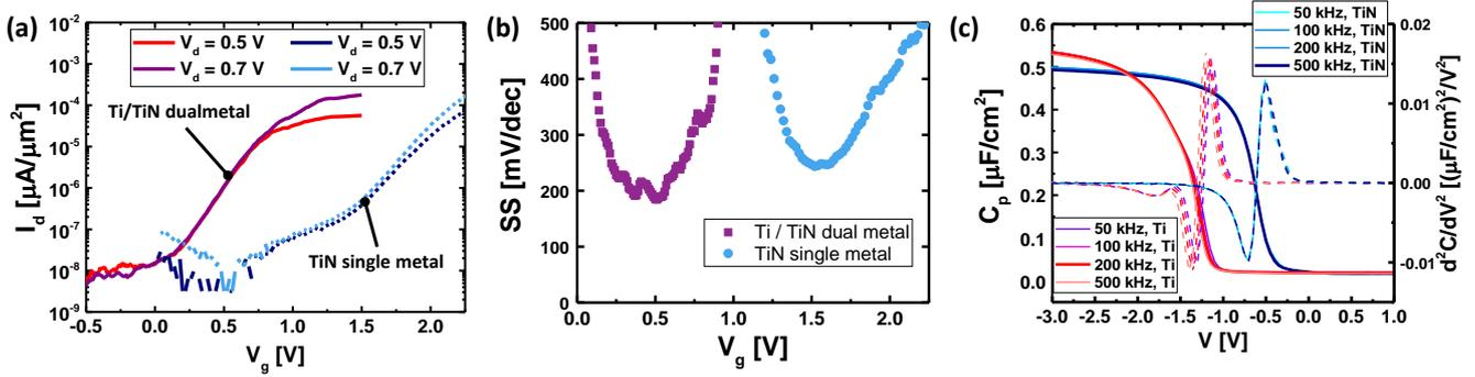
Fig. 2 (a) Transfer characteristics of devices with single (blue dashed lines) and dual-metal gates (red solid lines). The latter exhibits lower onset voltage and smaller  $SS_{\min}$  as evidenced in the SS vs.  $V_g$  plot (b). (c) Determination of the work function difference  $\Delta\Phi_m = \Delta V_{FB}$  with capacitance voltage measurements on Ti and TiN MOSCAPs.
