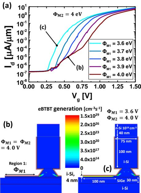
Fig. 3 (a) Simulated transfer characteristics emphasizing the necessity of using a dual metal gate to avoid a deteriorated subthreshold swing. In addition to a dual-metal gate, smaller EOT and thinner channel are required to boost the performance. (b) From eBTBT plots it becomes clear that premature tunneling into the pillar is the reason for the bipartite turn-on with a single gate-metal.
