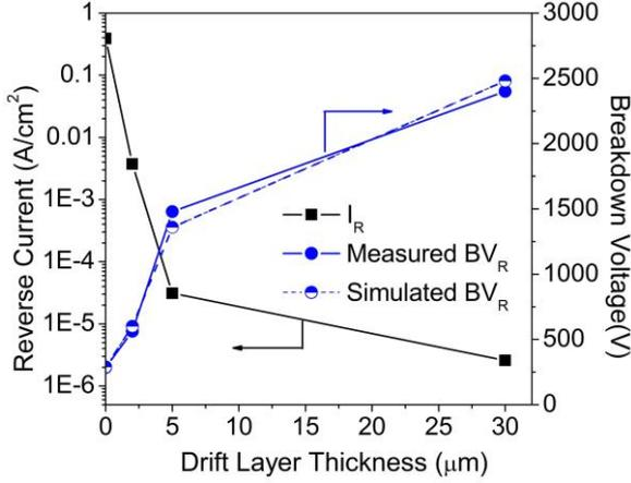
Figure 3: Reverse leakage current density, measured and simulated breakdown voltages for different DLT.
