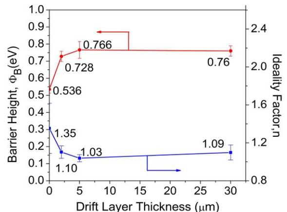
Figure 2: Schottky Barrier Height and Ideality Factor of vertical SBD (10 diodes) with different DLT on free-standing GaN.
