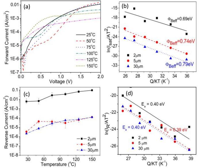
Figure 2: (a) Forward I-V-T characteristics of SBD with DLT of 2 $\mu\text{m}$ ; (b) Richardson's plot for forward current; (c) Reverse leakage current density (-20V) as a function of temperature; (d) Richardson's Plot for reverse leakage current.
