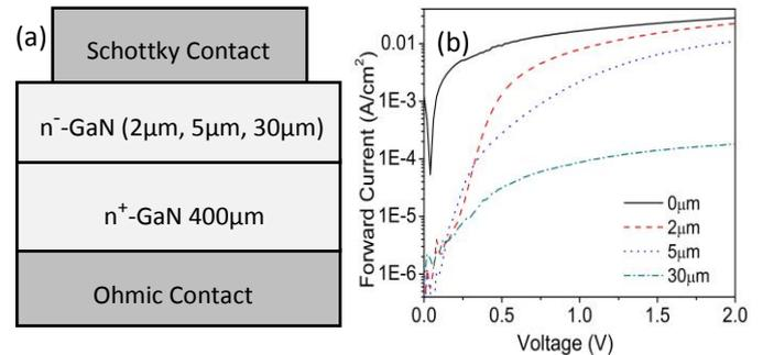
Figure 1: (a) Schematic cross-section of the fabricated vertical SBD on free-standing HVPE grown GaN with different drift layer thickness grown by MOCVD and (b) forward  $I$ - $V$  characteristics of vertical SBDs with different DLTs
