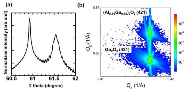
Fig. 1: (a) Symmetric HRXRD  $\theta$ - $2\theta$  scans for (020) diffraction of 240 nm  $\beta$ -(Al $_{0.16}$ Ga $_{0.84}$ ) $_2$ O $_3$ /Ga $_2$ O $_3$  (010) layers. (b) Symmetric on-axis (421) reciprocal space maps for the (AlGa) $_2$ O $_3$  layer on Ga $_2$ O $_3$  substrate.
