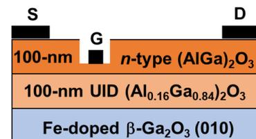
Fig. 2: Schematic cross section of Sn-doped  $\beta$ -(Al $_{0.16}$ Ga $_{0.84}$ ) $_2$ O $_3$  (010) channel MESFET.
