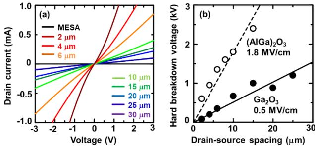
Fig. 3: Current-voltage characteristics of Sn-doped  $(\text{Al}_{0.16}\text{Ga}_{0.84})_2\text{O}_3$  with a donor concentration of  $2 \times 10^{18} \text{ cm}^{-3}$  for various contact resistances. (b) Two-terminal buffer-leakage breakdown voltage of unintentionally doped  $(\text{Al}_{0.16}\text{Ga}_{0.84})_2\text{O}_3$  (dash) and  $\text{Ga}_2\text{O}_3$  (solid) as a function of source-to-drain spacing.
