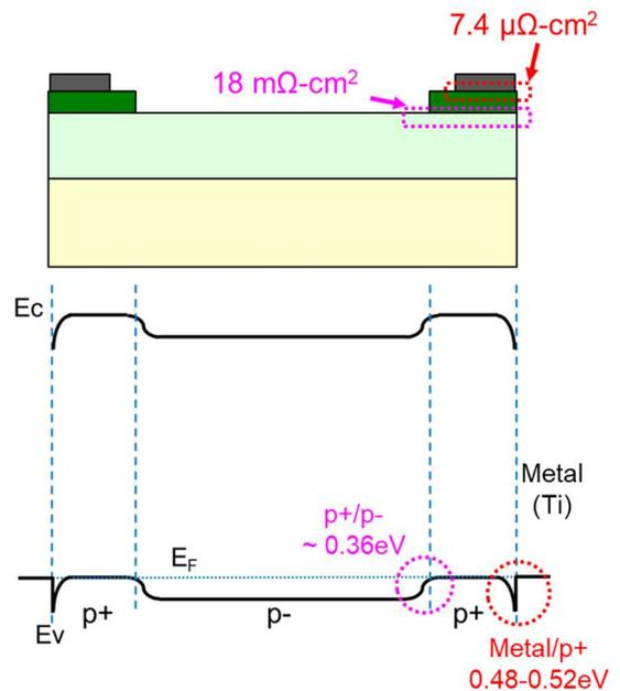
**Figure 3** Specific contact resistance of each interface.
