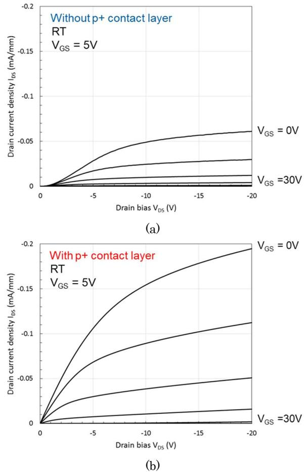
**Figure 2**  $I_{DS}$ - $V_{DS}$  characteristics of the diamond MESFETs (a) without p+ contact layer and (b) with p+ contact layer.
