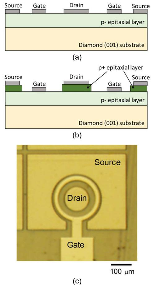
**Figure 1.** Cross sectional view of diamond MESFET structure. MESFET (a) without and (b) with p+ contact layer are fabricated onto identical sample. (c) Photograph of the MESFET structure (Corbino-shape).
