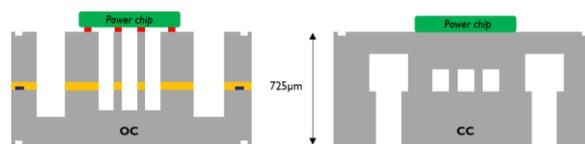
Fig. 1 - Open and close channels configurations.
