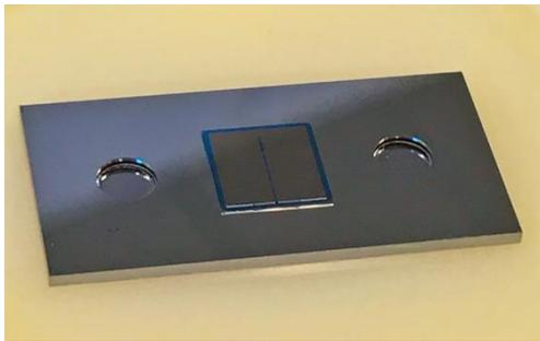
Fig. 3 – Photo of the final TCB between the OC and power test chips.
