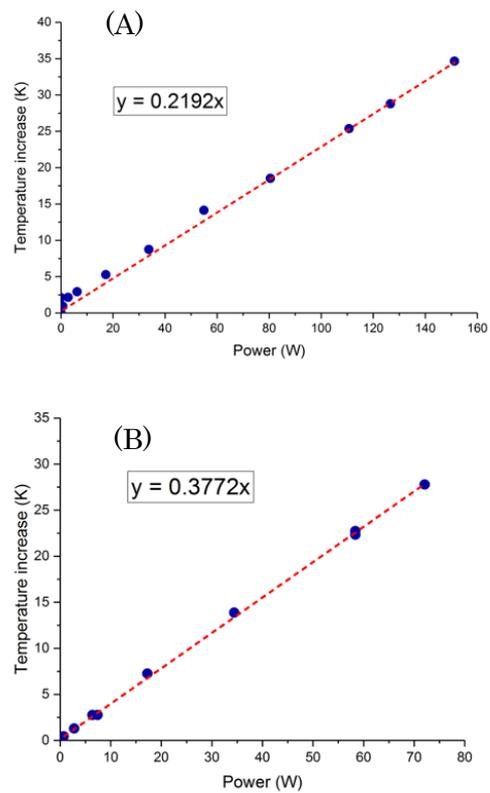
Fig. 4 – (A) Power test chip temperature increase when bonded to OC. A pressure of 1.8bar and a flow rate of 150ml/min are applied; (B) Power test chip temperature increase when bonded to CC. A pressure of 2.3bar and a flow rate of 143ml/min are applied.
