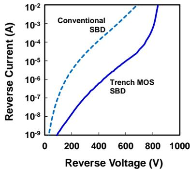
Fig. 2 Comparison of the reverse  $I$ - $V$  characteristics of a trench MOS SBD and a conventional SBD.
