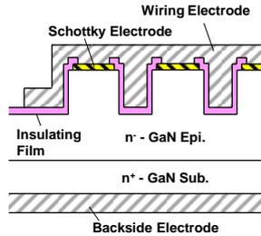
Fig. 1 Schematic cross section of the fabricated trench MOS SBD.
