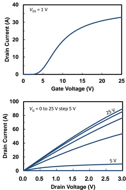
Fig. 5 Transfer  $I_D$ - $V_G$  and output  $I_D$ - $V_{DS}$  characteristics of a trench MOSFET chip with the chip resistance of 30 mΩ.
