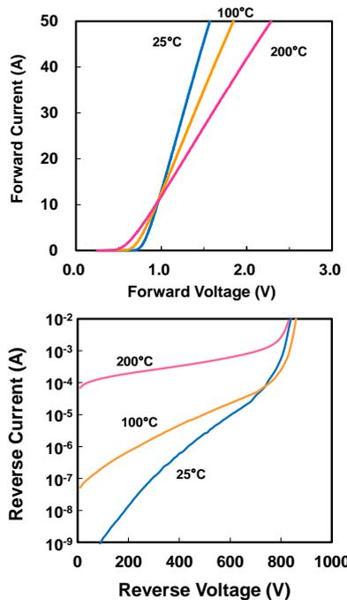
Fig. 3 Forward and reverse  $I$ - $V$  characteristics of the fabricated trench MOS SBD chips measured at 25, 100, and 200 °C.
