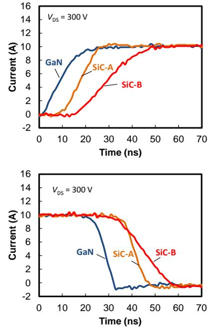
Fig. 4 Switching waveforms of resistive-load turn-on and turn-off operations for an 80-mΩ MOSFET chip.
