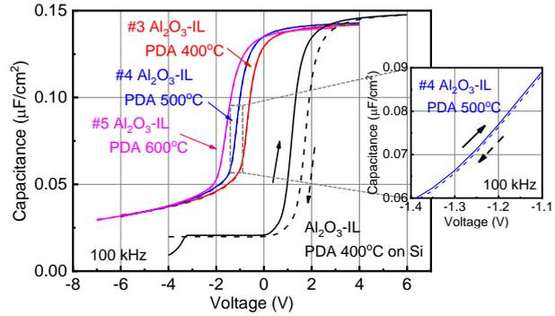
Fig. 3 Bi-directional  $C-V$  curves of 3C-SiC MOS capacitors with Al<sub>2</sub>O<sub>3</sub>-IL. Hysteresises of 3C-SiC MOSs are negligibly small.
