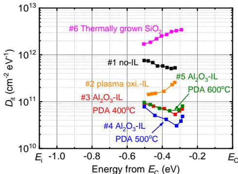
Fig. 5  $D_{it}$  distributions for 3C-SiC MOS capacitors in this study.
