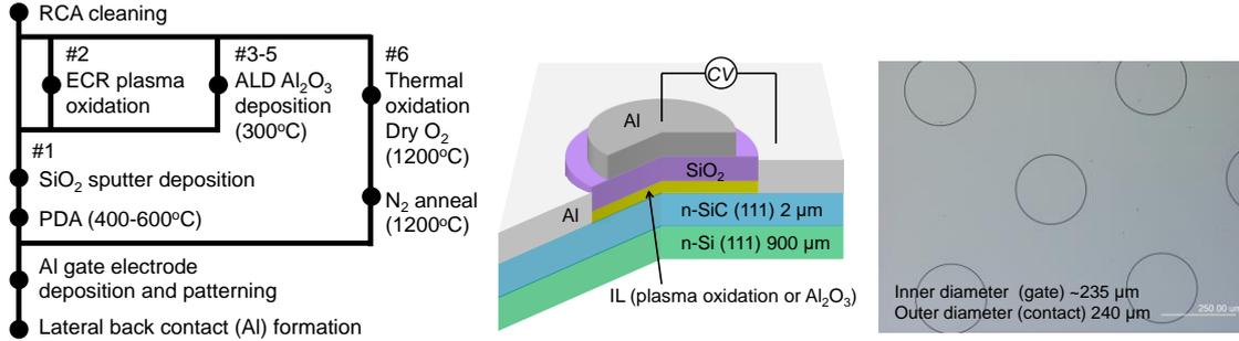
Fig. 1 Sample fabrication procedure, cross-sectional picture of fabricated lateral MOS capacitor, and top-view optical microscope image.
