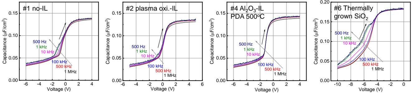
Fig. 4  $C-V$  frequency dependence for samples “#1 no-IL”, “#2 plasma oxidized-IL”, “#4 Al<sub>2</sub>O<sub>3</sub>-IL (PDA 500°C)”, and “#6 thermally grown SiO<sub>2</sub>”. Frequency range is 1 M – 500 Hz.
