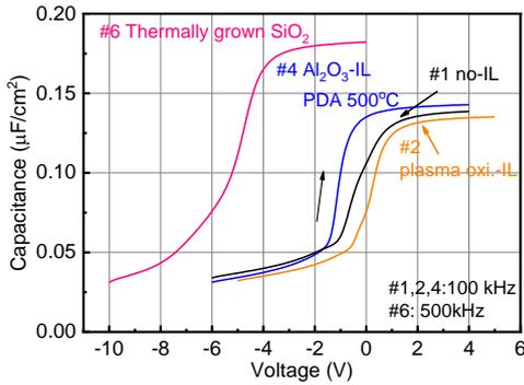
Fig. 2 High frequency  $C-V$  characteristics for 3C-SiC MOS capacitors with various structures.
