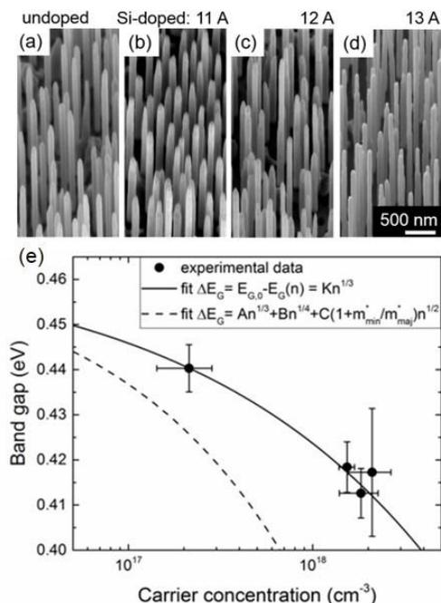
Figure 2. SEM images of undoped (a) and Si-doped (b-d) InAs NWs; (e) Band-gap as a function of n-type carrier concentration; best fit to the data gives the simple  $\Delta E_G = Kn^{1/3}$  law [5].
