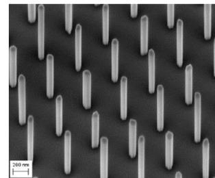
Figure 3. SEM image of Si-doped GaAs NWs grown by a non-VLS mechanism on Si(111) with high growth yield [7].
