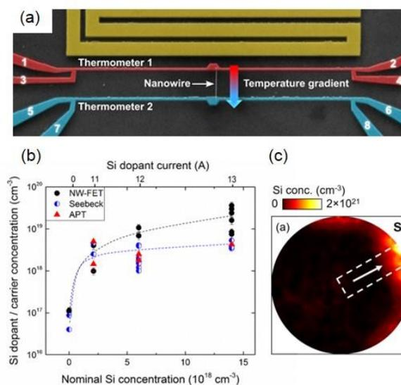
Figure 1. (a) SEM image of typical NW device for Seebeck effect measurement using lithographically defined heater and thermometers at both NW ends; (b) Comparison of bulk Si dopant concentration (APT data) and n-type carrier concentration (Seebeck and NW-FET data) as a function of nominal Si concentration; (c) APT reconstruction of a Si-doped InAs NW shown as projected 2D composition map, illustrating Si segregation at the NW sidewall surface [4].
