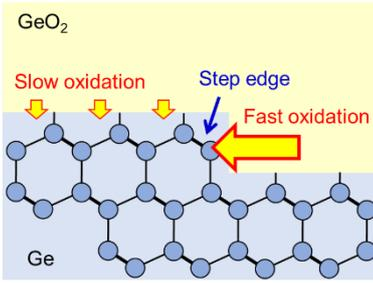
**Fig. 3** Schematic image of GeO<sub>2</sub> oxidation at GeO<sub>2</sub>/Ge(111) interface. The preferential step edge oxidation is simply described as different oxidation rate in direction to parallel to terrace from that in direction to perpendicular to terrace.
