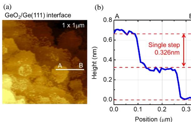
**Fig. 1** (a) AFM image of GeO<sub>2</sub>/Ge(111) interface oxidized at 550°C for 30 min. Clear step & terrace structure is observed. (b) Height profile between A and B points shown in (a). Single step height exactly corresponds to 2 atomic layers in Ge(111). Such a planarization in oxidation is never reported in Si.
