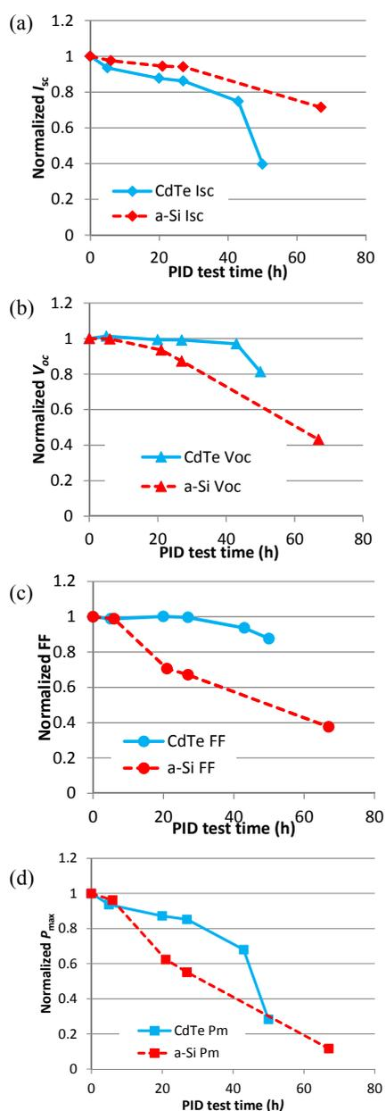
Fig. 1 Normalized  $I_{sc}$  (a),  $V_{oc}$  (b), FF (c) and  $P_{max}$  (d) for a-Si:H/ $\mu$ c-Si:H and CdTe PV modules as a function of PID test time.
