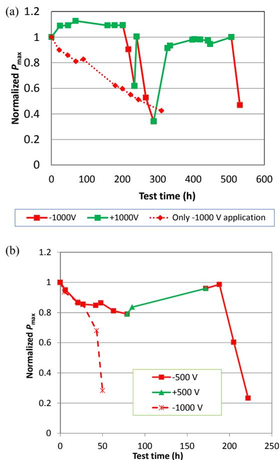
Fig. 2 Normalized  $P_{max}$  for a-Si:H/ $\mu$ c-Si:H (a) and CdTe (b) PV modules as a function of test time. Green and red symbols and guides for eye represent positive and negative voltage applications, respectively.
