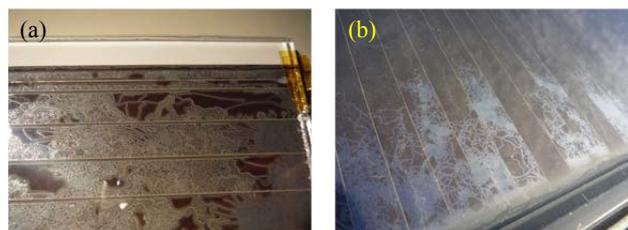
Fig. 3 Appearance of delamination observed for a-Si:H/ $\mu$ c-Si:H PV modules after indoor PID test (a) and outdoor exposure (b).
