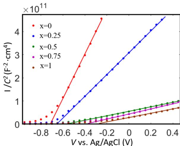
Fig.3 Mott-Schottky plot of  $\text{Fe}_{2-x}\text{Al}_x\text{O}_3/\text{TTO}$ . Electrolyte solution: 1 M NaOH.
