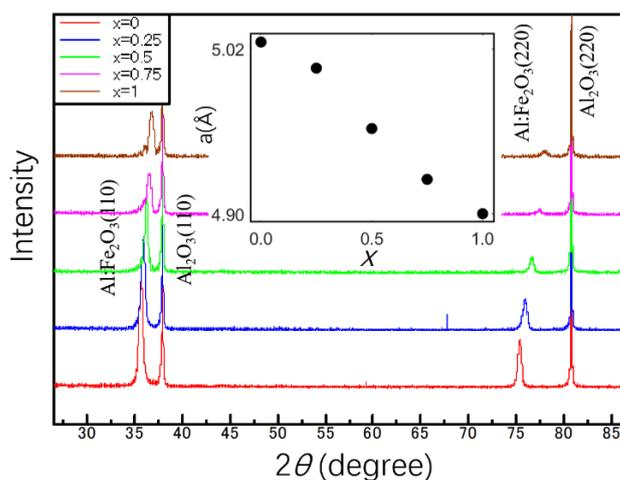
Fig. 1 XRD patterns of Fe<sub>2-x</sub>Al<sub>x</sub>O<sub>3</sub> films grown on Al<sub>2</sub>O<sub>3</sub> substrate with  $x$  values of 0, 0.25, 0.5, 0.75 and 1. The inset shows the compositional dependence of the lattice parameter  $a$ .
