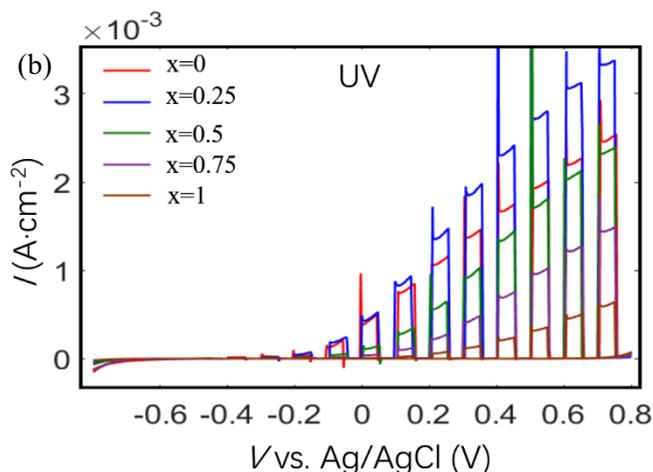
Fig. 2 Chopped  $I$ - $V$  curves under illumination with (a) vis light ( $\lambda=400$ - $700$  nm) and (b) UV light ( $\lambda=300$ - $400$  nm) for  $\text{Fe}_{2-x}\text{Al}_x\text{O}_3$  photoelectrodes.
