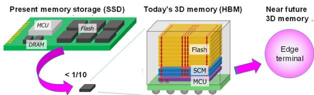
Fig. 1 A new concept of ultra-high density 3D storage memory system with ultrafine pitch TSVs for edge computing.
