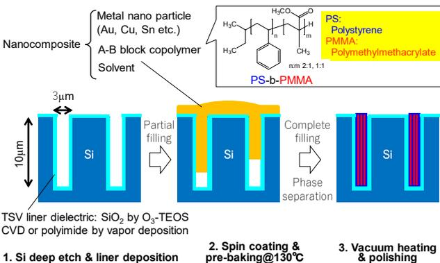
Fig. 3 A process flow for ultrafine pitch TSV formation based on DSA with nanocomposites consisting of metal nanoparticles and an A-B block copolymer.
