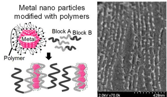
Fig. 6 Metal nano-cylinders resulted from a nanocomposite consisting of Au nanoparticles modified with a polymer.
