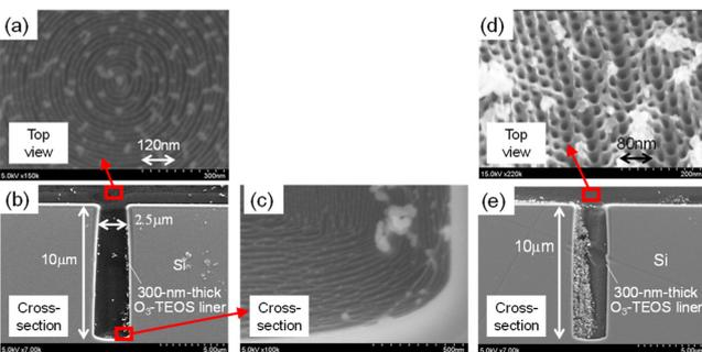
Fig. 4 SEM images of lamella (multiple annular) structure of PS-b-PMMA (1:1) in deep Si holes heated at 280C. Molecular weights of the PS/PMMA were 15,000/15,000 (a)-(c). SEM images of cylinder structure of PS-b-PMMA (2:1) in deep Si holes. Molecular weights of the PS and PMMA were 57,000 and 25,000 (d)-(e).
