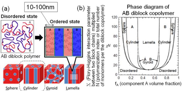
Fig. 2 Schematic illustration of typical nano-domain morphologies from an A-B block copolymer (a) and the block copolymer phase diagram (b).
