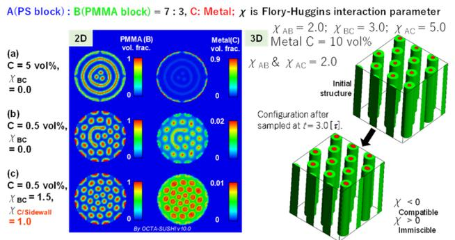
Fig. 5 2D (left) and 3D (right) morphology of PS-b-PMMA with metal in a deep Si hole calculated by the SCF theory.
