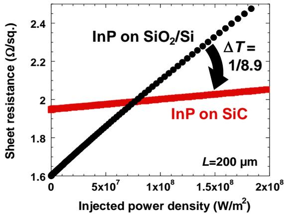
Fig. 4 Measured sheet resistance of resistance temperature detector on InP on SiC and InP on SiC wafers.
