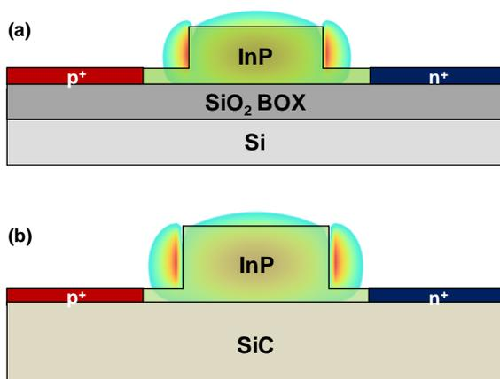
Fig. 1 (a) III-V on SiO<sub>2</sub>/Si platform and (b) III-V on SiC platform for photonic integrated circuits.
