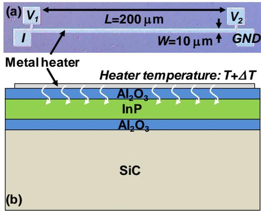
Fig. 3 Plan-view photo and cross-sectional schematic of resistance temperature detector on InP on SiC wafer.
