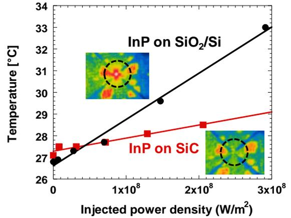
Fig. 5 Device temperature as a function of injected power density measured by thermal camera.
