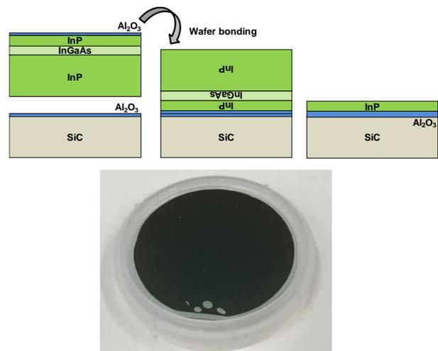
Fig. 2 Fabrication procedure and photo of III-V on SiC wafer.
