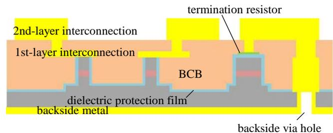
Figure 2 Schematic diagram of cross-sectional MZM integrated with termination resistor and backside via hole.
