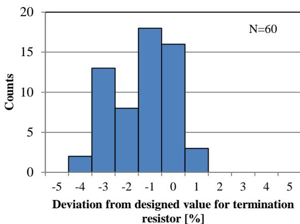
Figure 3 Histogram of deviation from designed value for termination resistor on a 4-inch diameter wafer.
