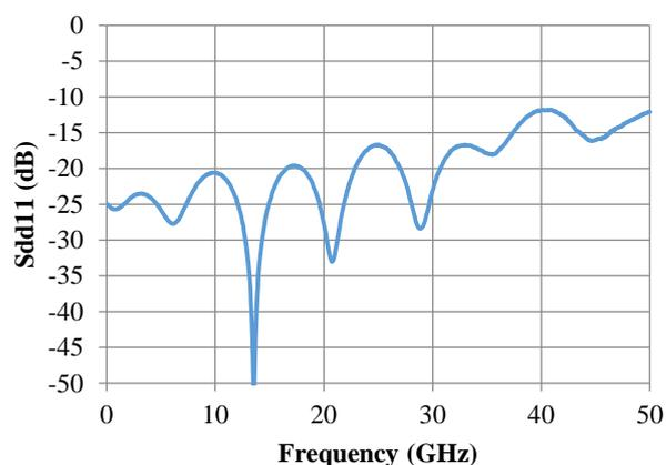
Figure 4 Differential small-signal frequency response for IQ-MZM integrated with RF termination resistor.
