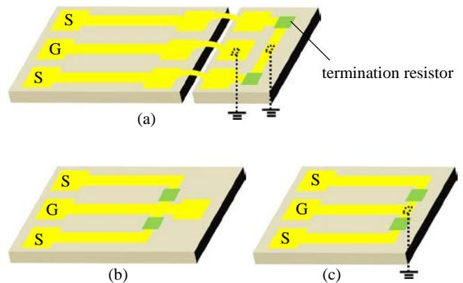
Figure 1 Schematic diagrams of (a) conventional optical device configuration using RF signals, (b) integration of termination resistors, (c) integration of termination resistors and backside via hole.
