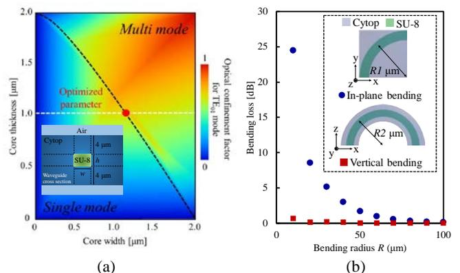
Fig. 2 (a) Calculated optical confinement factor of  $\text{TE}_{01}$  mode as a function of SU-8 core dimensions. Inset is cross section of waveguide; (b) In-plane and vertical bending loss at 90° bending as a function bending radius.
