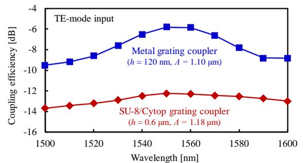
Fig. 5 Calculated TE-mode coupling efficiencies as a function of wavelength.
