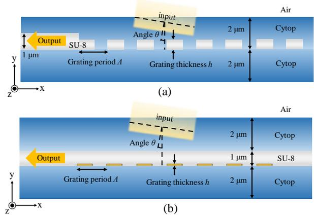
Fig. 3 Cross section of (a) SU-8/CYTOP grating coupler and (b) metal grating coupler. Light propagates in x direction in (a) and (b).
