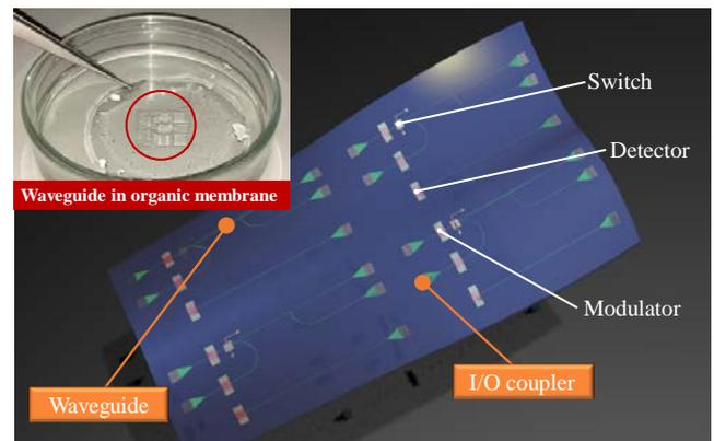
Fig.1 Schematic of organic-membrane PIC
