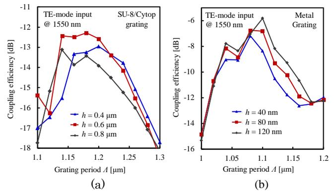
Fig. 4 Calculated TE-mode coupling efficiencies of (a) SU-8/CYTOP grating coupler and (b) metal grating coupler as a function of grating pitch  $A$ , with grating thickness  $h$  as a parameter.
