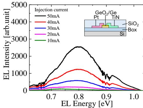
Fig. 3 EL spectra for GOI diodes.
