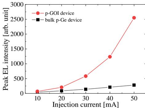
Fig. 4 Dependence of EL peak intensity on current intensity.
