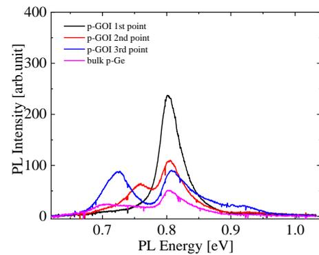
Fig. 5 PL spectra for bulk Ge and GOI substrates.
