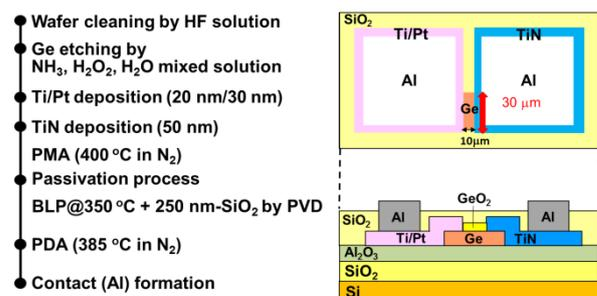
Fig. 1 Fabrication process flow, top and cross sectional views of device structure.
