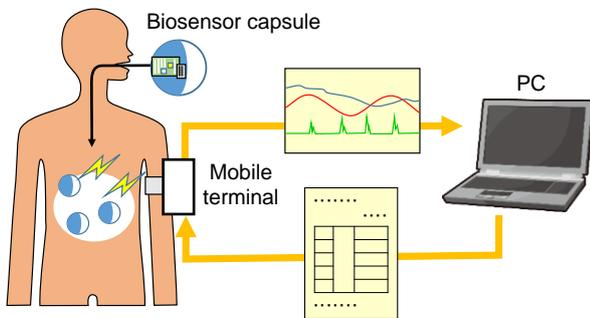
Fig. 1 An example of disposal biosensor for medical examination.
