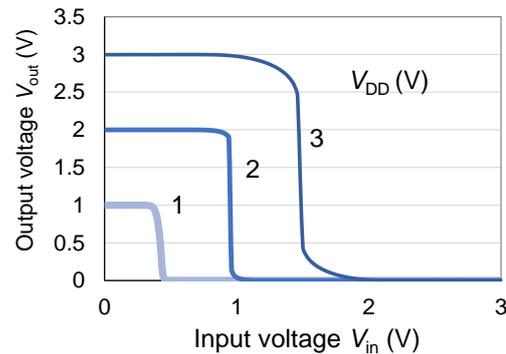
Fig. 5 Input and output characteristics of CMOS inverter.
