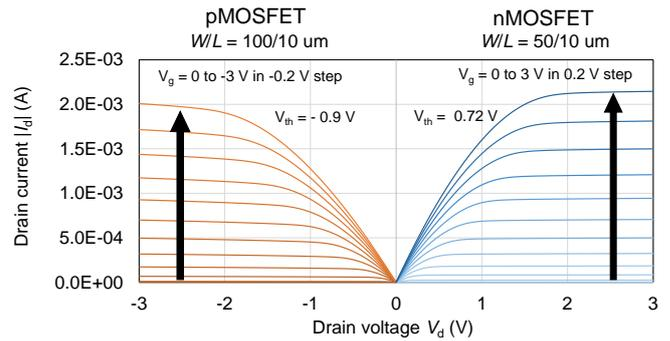
Fig. 4 Drain current ( $|I_d|$ ) vs. drain voltage ( $V_d$ ) characteristics for fabricated n-channel and p-channel MOS transistors.
