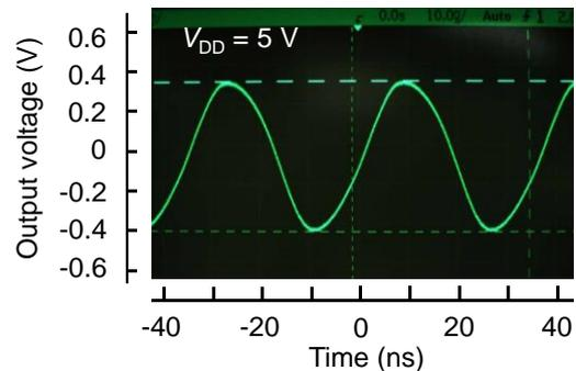
Fig. 6 Oscillation waveform of fabricated ring oscillator with three CMOS inverters.
