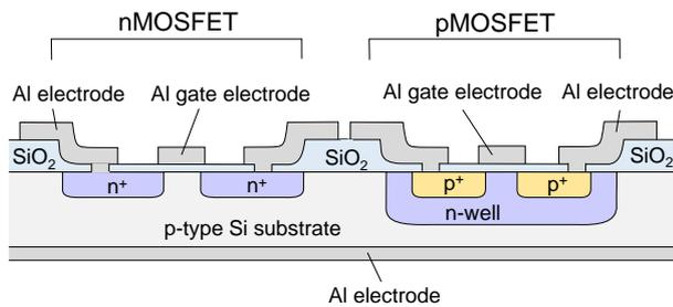
Fig. 2 Schematic structure of CMOS transistors.
