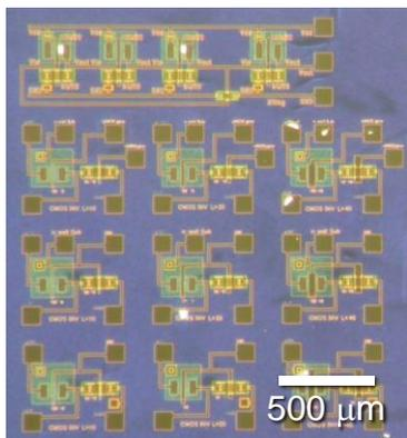
Fig. 3 Optical microscope image of part of the fabricated CMOS chip.
