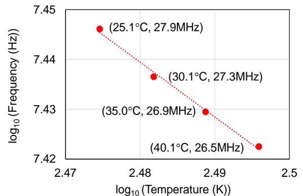
Fig. 7 Temperature dependence of oscillation frequency for the fabricated ring oscillator.
