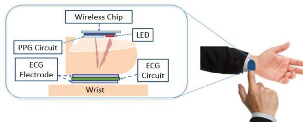
Fig. 1 Conceptual configuration of cuffless BP monitoring system
