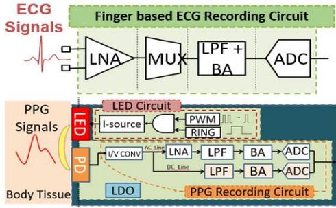
Fig. 2 Schematics of ECG and PPG circuits.
