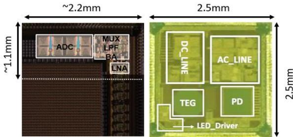
Fig. 3 Microphotographs of the fabricated ECG recording circuit (right) and PPG circuit (left) [6].
