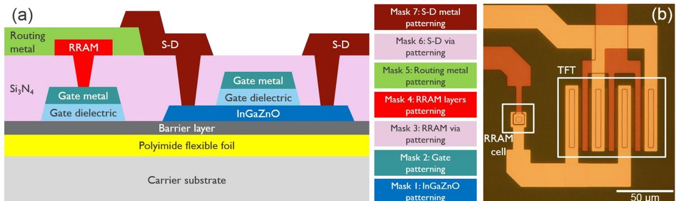
Figure 1. (a) Cross-section and mask set of TFT-RRAM device, (b) TFT-RRAM integration under 50x magnification
