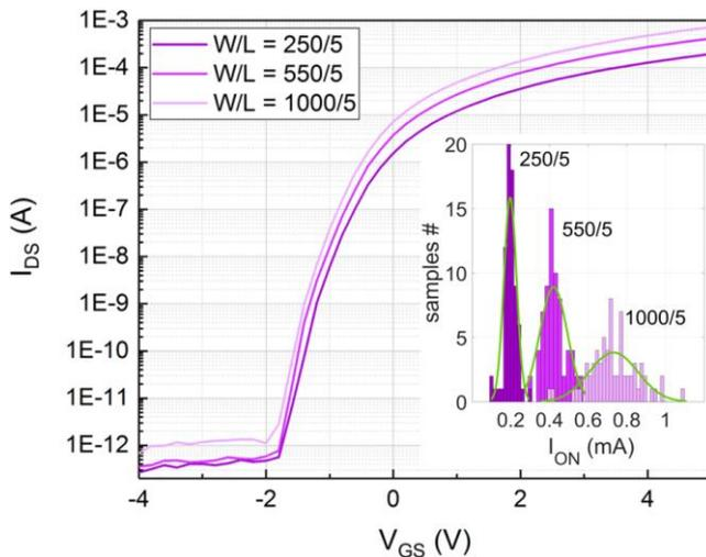
Figure 2. TFT transfer characteristics for different TFT sizes:  $W/L = 250/5$ ,  $W/L = 550/5$ ,  $W/L = 1000/5$
