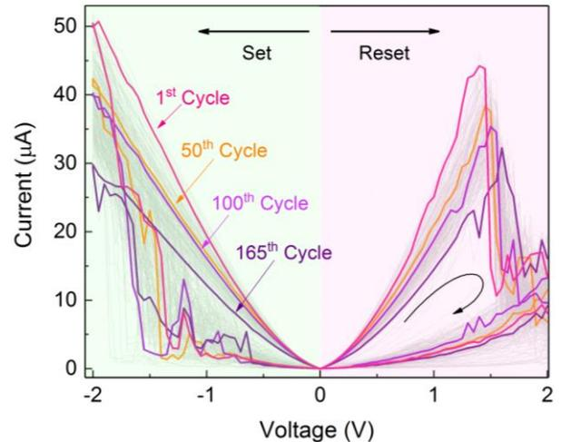
Figure 4. TFT-RRAM switching characteristics based on 165 cycles
