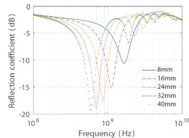
Fig. 3. Relation of frequency and the reflection coefficient when the thickness of the fat is between 8 mm and 40 mm.
