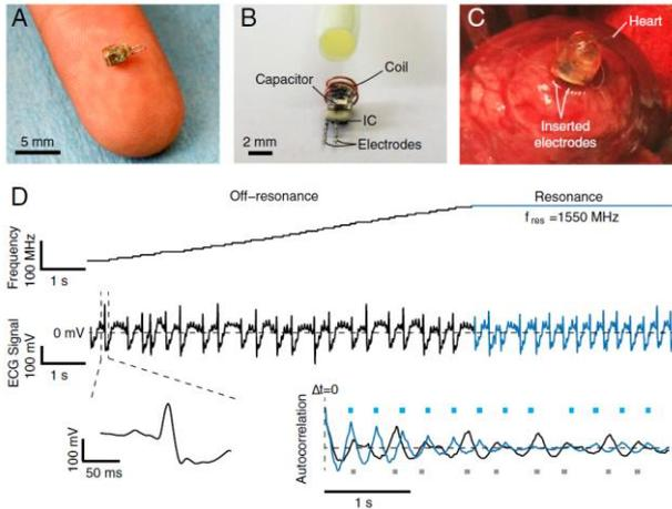
Fig. 2. (a) Electro-stimulator on a finger (b) Zoomed-in view of the device (c) device implanted on the heart of a rabbit (d) Operating frequency variation from the off-resonance to the resonant frequency (top). Measured ECG of the rabbit corresponding to the operating frequency variation (middle). The autocorrelation (bottom) shows that the neuro-stimulator makes the heart beat regular when enough power is wirelessly supplied.
