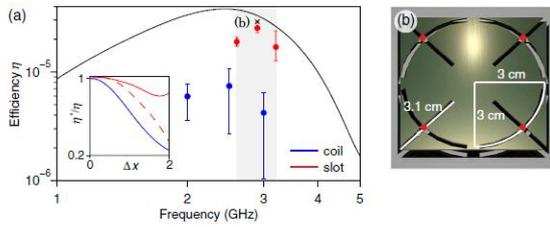
Fig. 1. (a) Theoretical upper bound on efficiency (black curve) with efficiencies of the slot array (red) and the coil sources (blue) (b) physical dimension of the slot array.
