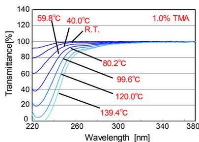
Fig. 4 Change in transmission spectrum of 1.0%TMA at elevated temperature.
