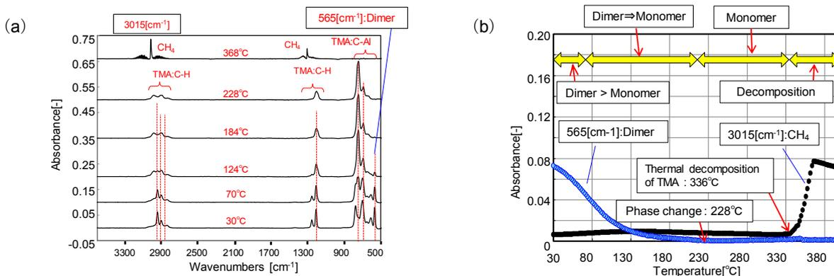
Fig. 5 (a) IR Spectral change of TMA at elevated temperature. (b) IR Absorbance change of TMA at elevated temperature.
