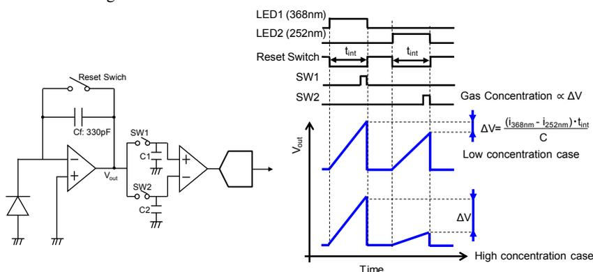
Fig. 3 The charge amplifier based photodetector circuit and timing diagram for signal sampling (Using time-sharing dual wavelength UV light absorption method).
