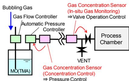
Fig. 1 Targeted MO gas supply system with gas concentration sensor.
