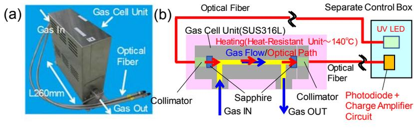
Fig. 2 (a) Picture and (b) schematic diagram of fabricated gas concentration sensor.
