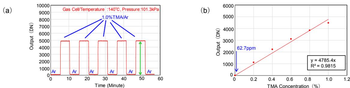
Fig. 6 (a) Fluctuation in output value of the concentration sensor unit when 1% TMA and 100% Ar were switched and (b) TMA concentration calibration curve.
