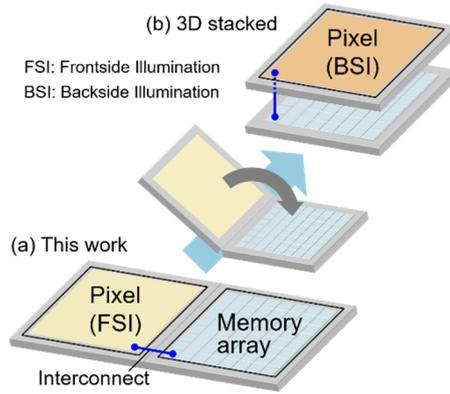
Fig. 2 Conceptual illustrations of pixel arrangement of (a) this work and (b) 3D stacked chip.
