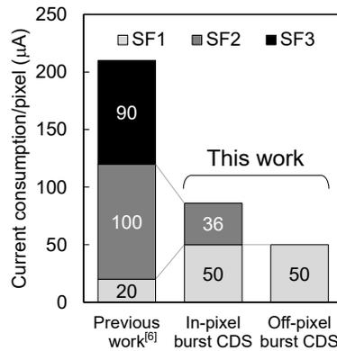
Fig. 7 Current consumption/pixel during video capturing.
