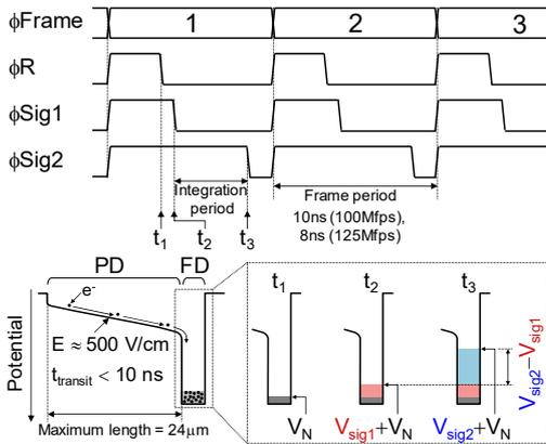
Fig. 6 Pulse timing diagram of burst CDS and pixel potential diagram.
