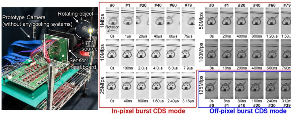
Fig. 9 Sample video capturing system and captured images at various frame rate.
