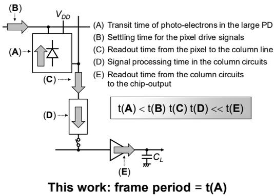
Fig. 1 Limiting factors of frame rate in CMOS image sensors.
