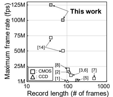
Fig. 8 Frame rate as a function of record length.
