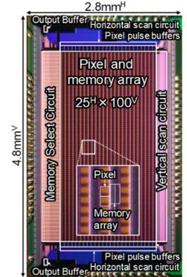
Fig. 3 Chip micrograph and block diagram.
