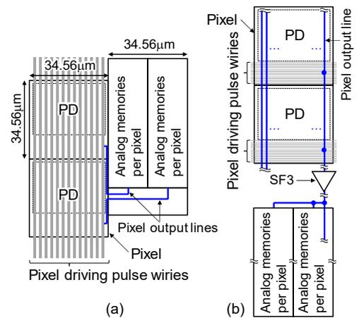
Fig. 5 Pixel layout diagram of (a) this work and (b) previous works[3,6].
