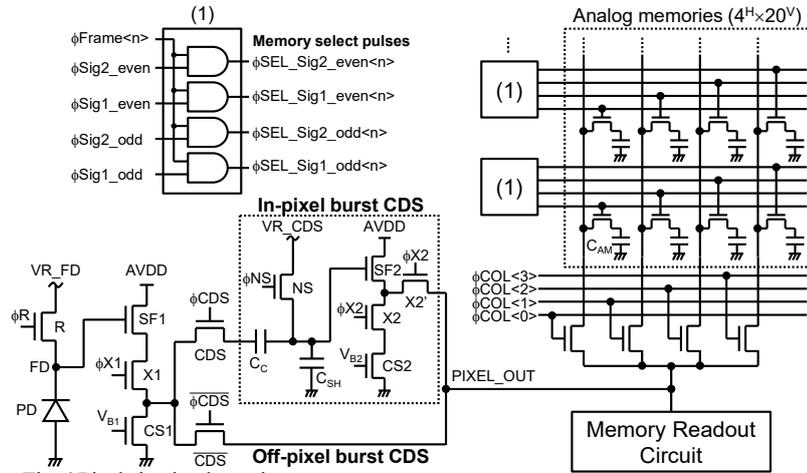
Fig. 4 Pixel circuit schematic.
