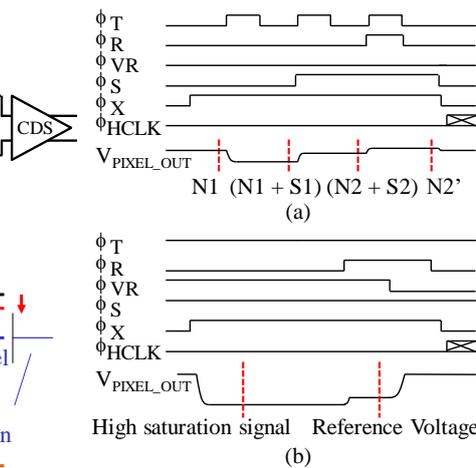
Fig. 3 Timing diagrams in H blanking period of (a) the wide dynamic range LOFIC S1 & S2 operation and (b) the Dual VR high SNR absorption imaging operation.
