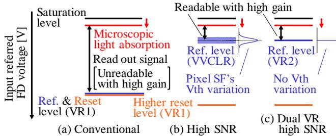
Fig. 2 Conceptual diagram of the three operation modes.
