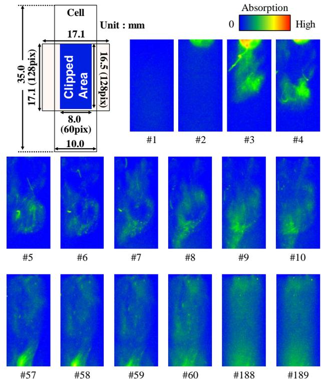
Fig. 9 Diffusion of 0.96ppm ozonated water visualized by 254nm light wavelength absorption imaging.
