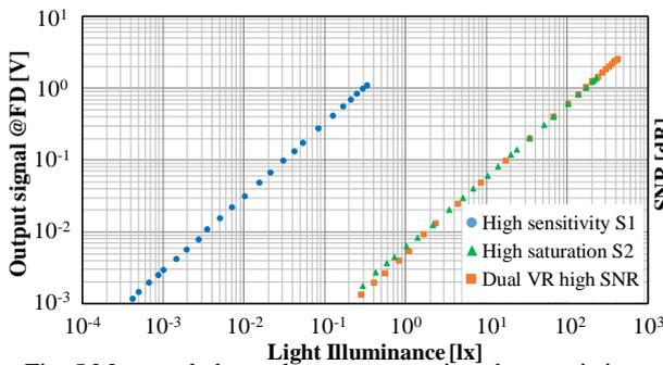
Fig. 5 Measured photo-electron conversion characteristic.
