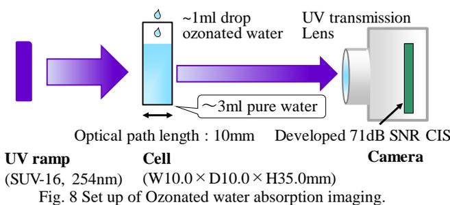
Fig. 8 Set up of Ozonated water absorption imaging.
