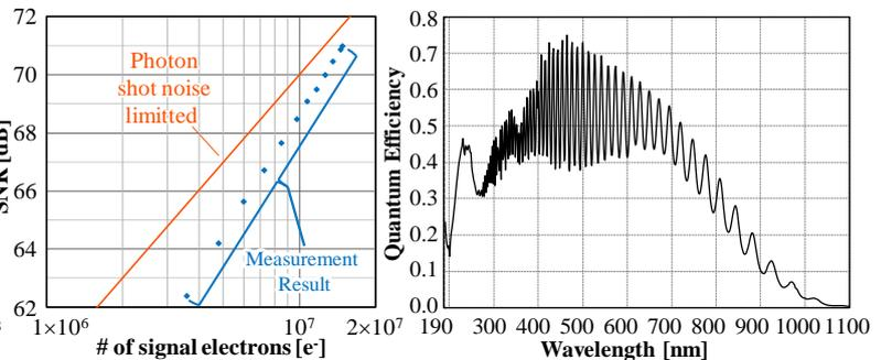
Fig. 6 Measured photon transfer curve in dual VR high SNR mode.
