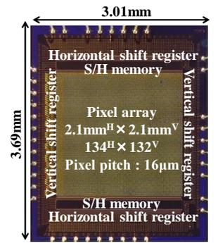
Fig. 4 micrograph of the developed CIS chip.
