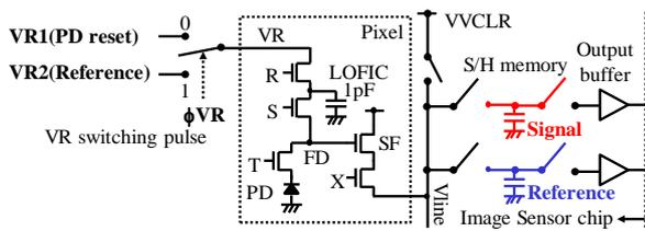
Fig. 1 Circuit architecture of the developed CIS.
