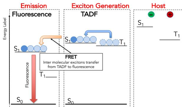
Fig.1 Mechanism of Hyperfluorescence™
