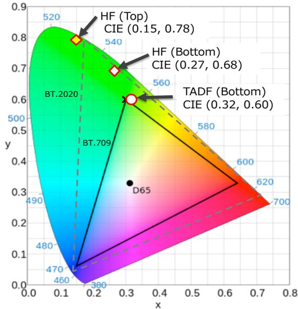
Fig.5 Comparisons of CIE xy of TADF-BE, HF-BE and HF-TE
