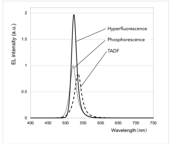
Fig.6 EL Spectrums of Phosphorescence, TADF and HF
