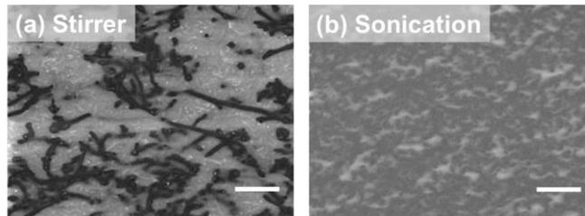
Fig. 3 SEM image of the surface of the printed 4 wt% MWCNT-filled copolymers fabricated by (a) stirrer and (b) sonication. The scale bar corresponds to 10 μm.
