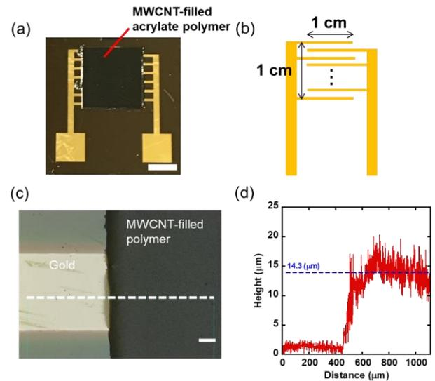
Fig. 1 Printed temperature sensor (8 wt% MWCNT-filled polymer by sonication process). (a) The picture of the temperature sensor. The scale bar corresponds to 5 mm. (b) Structure of interdigit electrodes.  $W/L = 1 \text{ cm} / 400 \mu\text{m}$ . (c) Optical image of the device. The scale bar corresponds to  $100 \mu\text{m}$ . (d) Height profile of the temperature sensor corresponding to the dashed white line of panel (c).
