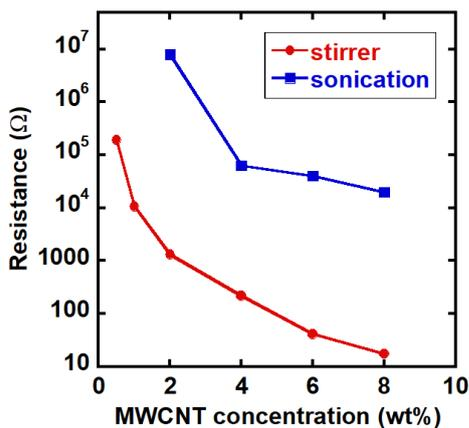
Fig. 2 The relation between electrical resistance and MWCNT content for the MWCNT/acrylate polymer composites fabricated by stirrer or sonication, respectively.
