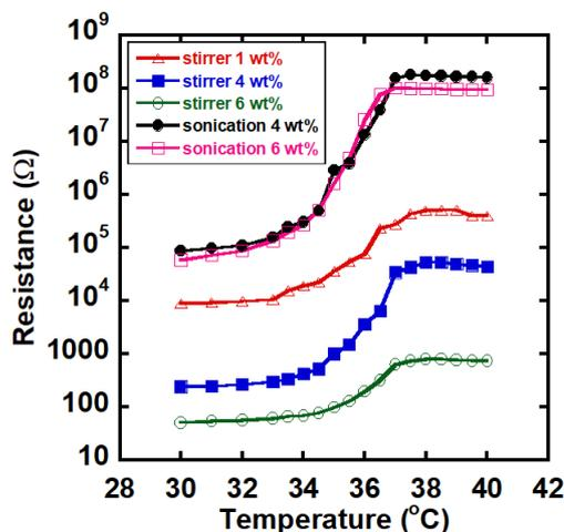
Fig. 4 The effect of temperature on the electrical resistance of various polymer composites; 1, 4, or 6 wt% MWCNT-filled polymer composites fabricated by stirrer and 4 or 6 wt% MWCNT-filled polymer composites by sonication.
