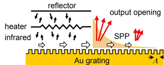
Fig. 1: Schematic drawing for showing the principle of the wavelength selective emission propagated through SPP.
