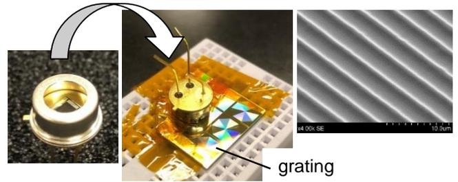
Fig. 5: Setup for observing the wavelength selectivity using the blackbody emitter on the fabricated grating.
