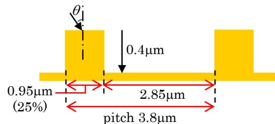
Fig. 2: Grating design based on 2D model.
