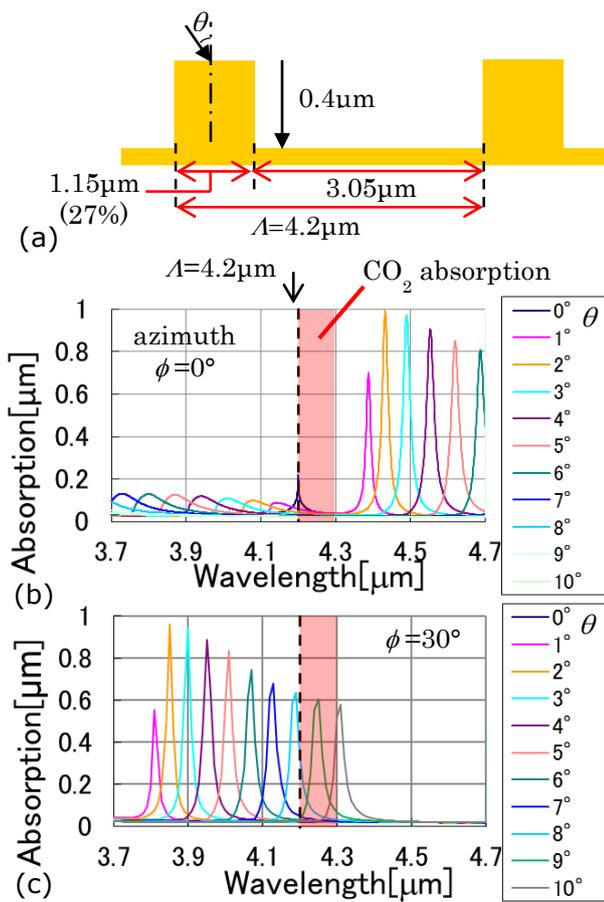
Fig. 4: (a) Grating design based on 3D model. (b) Simulated SPP related peaks when azimuth  $\phi$  is (b)  $0^\circ$  and (c)  $30^\circ$ . The legend shows the polar angle.
