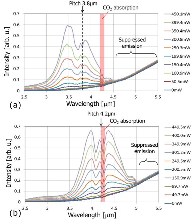
Fig. 6: FT-IR spectra of the emission using the commercially available blackbody emitter. The gratings are designed based on (a) 2D and (b) 3D models.
