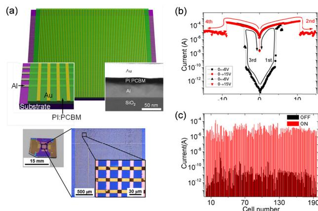
Fig. 1. (a) Schematic and images of  $64 \times 64$  array (4 Kbit) microscale organic memory devices. (b) Representative memory data. (c) Cumulative probability of ON and OFF states from 195 measured memory cells. Results from Ref. [5].
