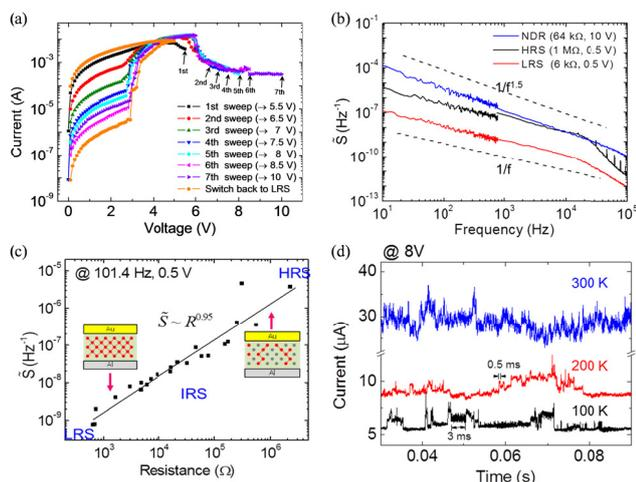
Fig. 2. (a) Intermediate resistance states. (b)  $1/f$  noise analysis of organic nanocomposite memory. (c) Scaling behavior between relative power spectral density and resistance. (d) Telegraphic fluctuation is reduced at lower temperature and lower applied bias. Results from Ref. [7,8].
