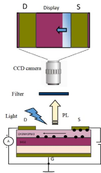
Fig. 1 Experiment setup for PL decay imaging
