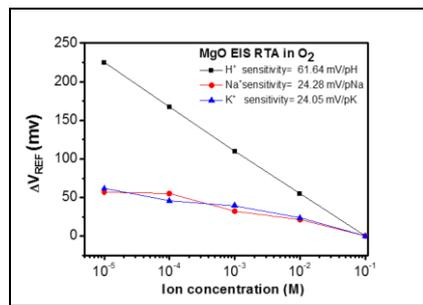
Fig. 10 The different ion sensitivity of MgO sensing membrane annealed 800°C in O<sub>2</sub> ambient
