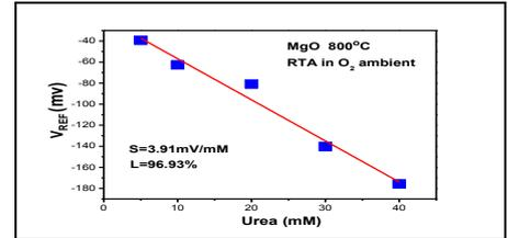
Fig. 12 pUrea-response of enzyme-immobilized MgO annealed at 800°C in O<sub>2</sub> ambient
