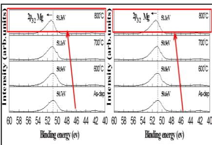
Fig. 5 XPS results of MgO film (a) Mg 2p in O<sub>2</sub> ambient (b) Mg 2p in N<sub>2</sub> ambient
