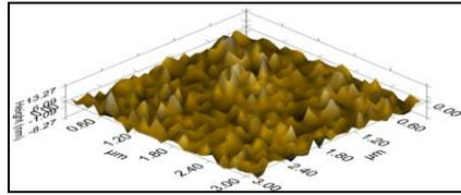
Fig. 7 AFM of high-k MgO surface after RTA at 800°C in N<sub>2</sub> R<sub>rms</sub>=2.85 (nm)
