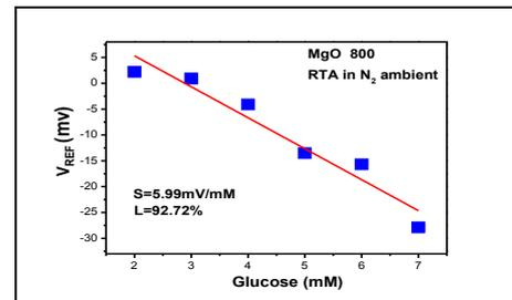
Fig. 15 pGlucose-responses of enzyme-immobilized annealed at 800°C in N<sub>2</sub> ambient
