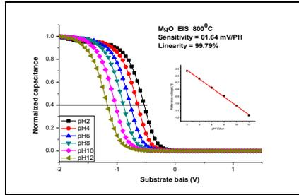
Fig. 8 The normalized C-V curve of MgO sensing membrane with RTA at 800°C in O<sub>2</sub>, the inset figure represents the sensitivity and linearity
