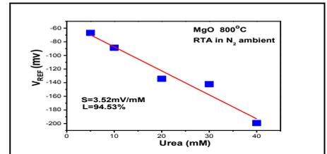
Fig. 13 pUrea-response of enzyme-immobilized MgO annealed at 800°C in N<sub>2</sub> ambient
