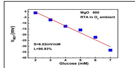
Fig. 14 pGlucose-responses of enzyme-immobilized annealed at 800°C in O<sub>2</sub> ambient
