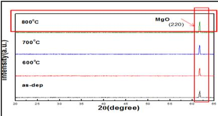
Fig. 3 XRD of the MgO film after annealing at various temperatures on single crystalline silicon in N<sub>2</sub> ambient for 30 sec
