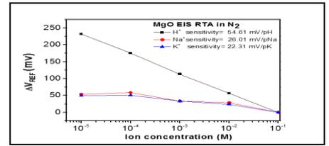
Fig. 11 The different ion sensitivity of MgO sensing membrane in N<sub>2</sub> ambient
