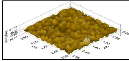
Fig. 6 AFM of high-k MgO surface after RTA at 800°C in O<sub>2</sub> R<sub>rms</sub>=4.33(nm)
