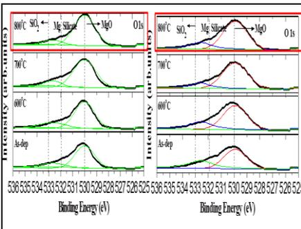
Fig. 4 XPS results of MgO film (a) O 1s in O<sub>2</sub> ambient, (b) O 1s in N<sub>2</sub> ambient
