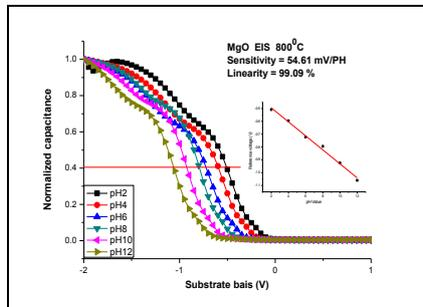
Fig. 9 The normalized C-V curve of MgO sensing membrane with RTA at 800°C in N<sub>2</sub>, the inset figure represents the sensitivity and linearity
