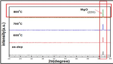
Fig. 2 XRD of the MgO film after annealing at various temperatures on single crystalline silicon in O<sub>2</sub> ambient for 30 sec
