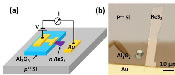
Fig. 2 (a) Schematic diagram of Si-ReS<sub>2</sub> *p-n* junction diode. (b) Optical image of the fabricated device.
