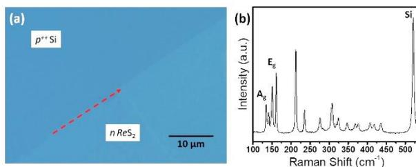
Fig. 1 (a) Optical image of Si-ReS<sub>2</sub> *p-n* junction formation. Red arrow shows the interface. (b) Raman spectra of the few-layer ReS<sub>2</sub> sample.
