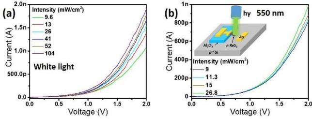
Fig. 4 (a,b)  $I$ - $V$  characteristics of the  $p$ - $n$  diode under different intensity of incident white light and 550 nm light illumination, respectively. Inset in Fig. 4(b) shows the schematic of photocurrent measurements during global irradiation of light without focusing through lens.
