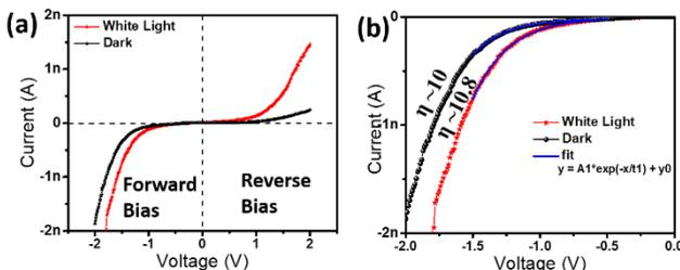
Fig. 3 (a) *I-V* characteristics of the fabricated *p-n* junction with and without white light illumination. (b) Forward bias *I-V* characteristics are fitted with forward bias diode equation.
