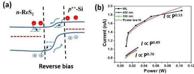
Fig. 5 (a) Schematic band diagram of Si-ReS<sub>2</sub>  $p$ - $n$  junction diode under reverse bias operation. Bulk trap states, interface trap states and defects levels are shown by dashed lines. (b) Power dependence current at reverse bias of 2 V under different light power and wavelength of illumination.
