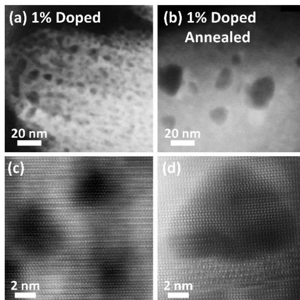
Fig. 1 HRTEM images of Sb-doped ZnO nanowires before and after annealing.
