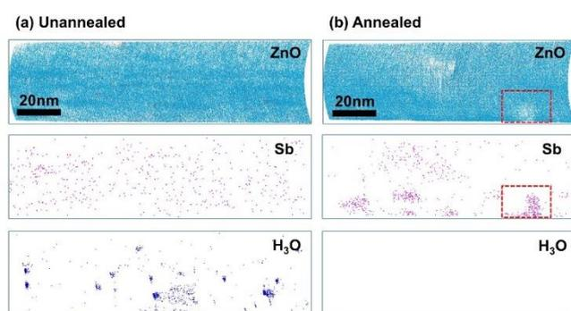
Fig. 2 Atom probe tomography scans of Sb doped ZnO nanowires before and after annealing.
