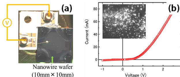
**Fig. 5.** Nanowire LED device and electrical performance. (a) Nanowire sample attached on a ceramic substrate. (b) Typical I-V curve. The inset shows an EL image taken by an infrared CCD camera in Micro-PL system ( $\times 20$  lens). The image area is  $380 \mu\text{m} \times 475 \mu\text{m}$ .
