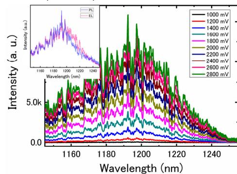
**Fig. 7.** EL spectra of the nanowire shown in Fig. 6 with increasing bias (step: 0.2 V). The inset shows PL and EL at 2.8 V bias, indicating good agreement of two peaks.
