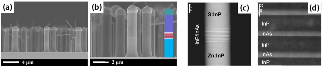
**Fig. 1.** (a) and (b) SEM images of vertically aligned InP/InAs nanowires. The inset in (b) shows schematic diagram of the p-i-n structured nanowire. (c) and (d) HAADF-STEM image of a nanowire with 10 InAs active layers.
