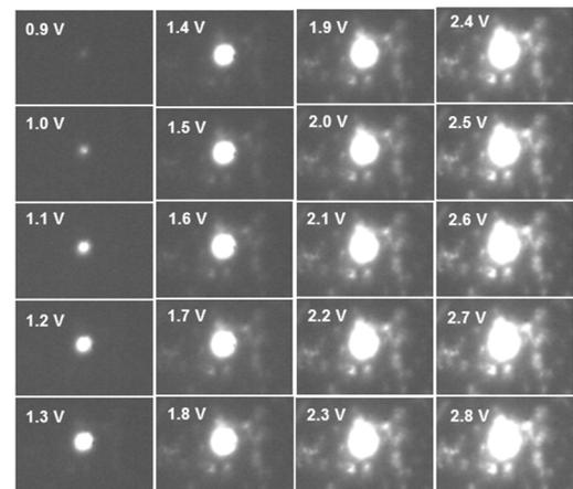
**Fig. 6.** EL images of a same single nanowire under bias voltage shown inside. Images were taken by an infrared CCD camera in Micro-PL system ( $\times 50$  lens). Each image area is  $47.6 \mu\text{m} \times 68.5 \mu\text{m}$ .
