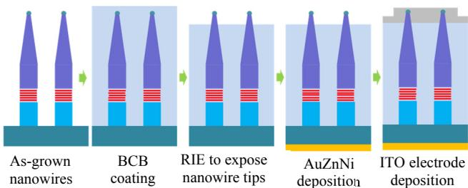
**Fig. 3.** Schematic diagram of device fabrication for nanowire LED. Nanowires were embedded in transparent BCB polymer material.
