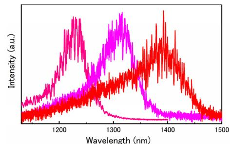
**Fig. 8.** EL spectra of three nanowire LED samples with increasing thickness of InAs layers modulated by flow rates of source materials of TMIn and TBAs.
