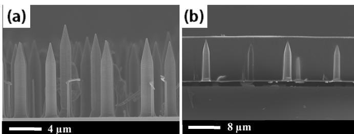
**Fig. 4.** Cross-section SEM images of (a) InP/InAs nanowires with tiny indium particles at tips after growth and (b) nanowire LED with nanowires embedded into BCB material.
