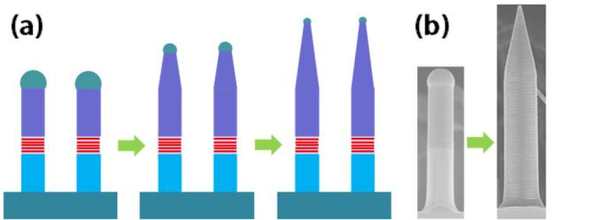
**Fig. 2.** Schematic diagram (a) and SEM images (b) of tuning indium particle into sub-100-nm diameter by modulating V/III ratio.
