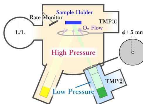
Fig. 1 Differential-pressure-type deposition chamber.
