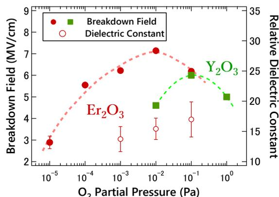
Fig. 2 Breakdown field and dielectric constant vs  $P_{\text{O}_2}$ .
