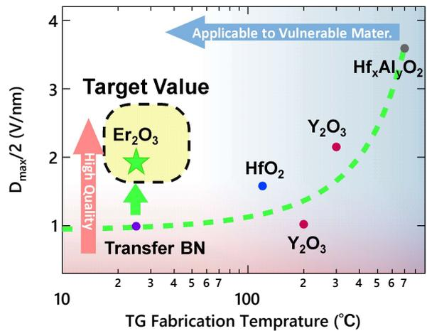
**Fig. 6**  $D_{\text{max}}$  as a function of the deposition temperature for high- $k$  on graphene. The literature data in which the defects are introduced in graphene are omitted here.
