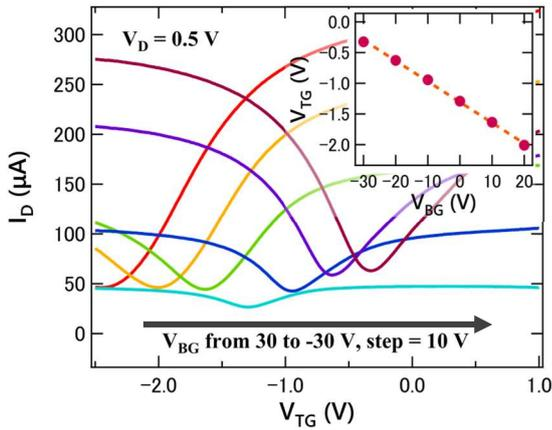
**Fig. 3**  $I$ - $V$  curves as a function of  $V_{TG}$ . The inset represents the Dirac point shift as a function of  $V_{BG}$ .
