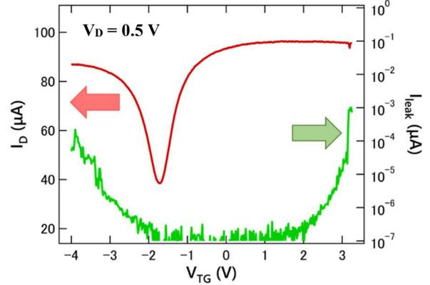
**Fig. 5**  $I_D$ - $V_{TG}$  curve and  $I_G$ - $V_{TG}$  at  $V_{BG} = 0$  V for 3.6-nm  $\text{Er}_2\text{O}_3$  top gate graphene FET.
