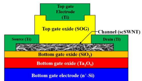
Fig. 1 Schematic structure of fabricated double-gate scSWCNT-TFT with engineered gate oxide.
