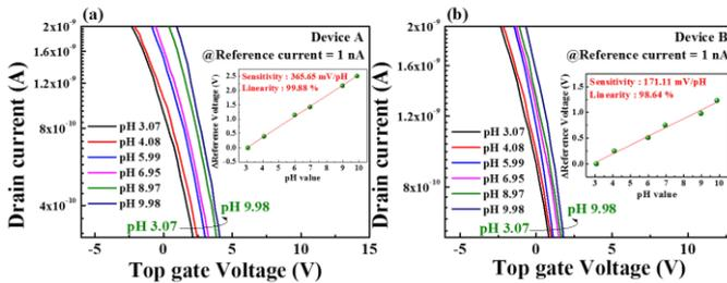
Fig. 2 Transfer characteristic curves of the double-gate structure scSWCNT TFTs for (a) Device A and (b) Device B at various pH buffer solutions.
