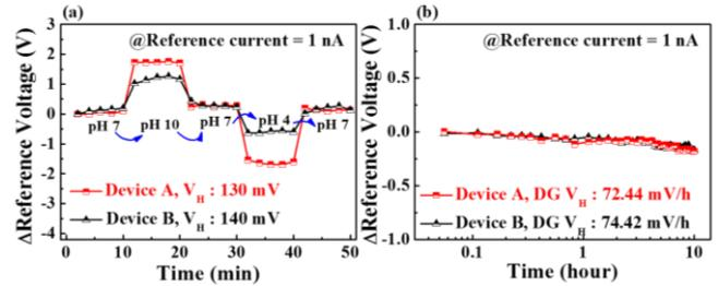
Fig. 3 (a) Hysteresis effect and (b) drift effects of the double-gate structure CNT TFTs with different bottom-gate oxide.
