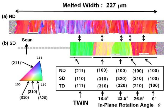
Fig. 2. EBSD maps at a high laser power. (a) IPF ND and (b) IPF SD. The crystal orientations are analyzed and shown in the inserted table. The SiO<sub>2</sub> cap thickness was 84 nm,  $P(I-R) = 1.14$  W.
