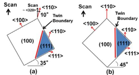
Fig. 4. Generation model of the (211) ND texture shown in Fig. 3. Firstly the rotated crystals are grown at rotation angles of (a) 35° or (b) 45° around the (100) ND and secondary twins are formed by the rotation of the solidified crystals on the (111) planes.
