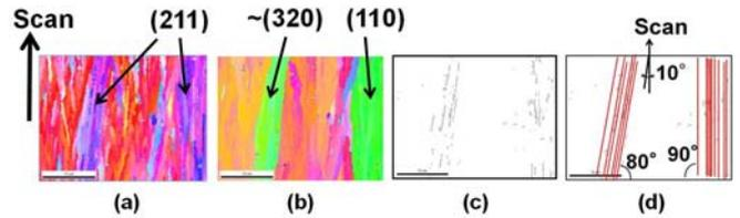
Fig. 3. EBSD maps at the center of melted width crystallized at a high laser power. (a) IPF ND, (b) IPF SD, (c) twin boundaries and (d) lines to delineate the tilt angles of twin boundaries. The SiO<sub>2</sub> cap thickness was 183 nm and  $P(I-R) = 1.47$  W.
