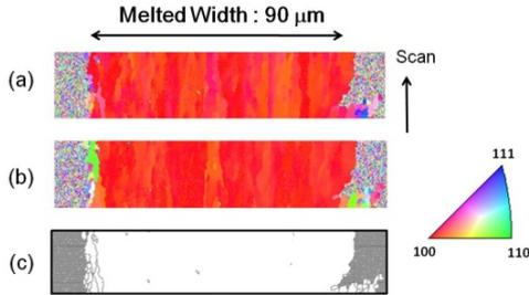
Fig. 1. EBSD maps at a low laser power close to the threshold of lateral grain growth. (a) IPF ND, (b) IPF SD, and (c) Grain boundary having rotation angle between 15-65°. The SiO<sub>2</sub> cap thickness was 123 nm and  $P(I-R) = 1.05$  W.
